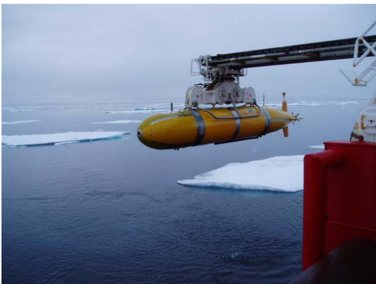
The Autosub autonomous underwater vehicle being launched from RRS James Clark Ross (Photo: Ken Collins, NOCS)
