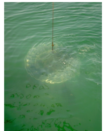
CTD rosette water sampling in the green eutrophic waters of the Gulf of Oman
