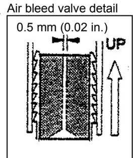
**Note:** Periodically clean air bleed valve to ensure proper functioning.
