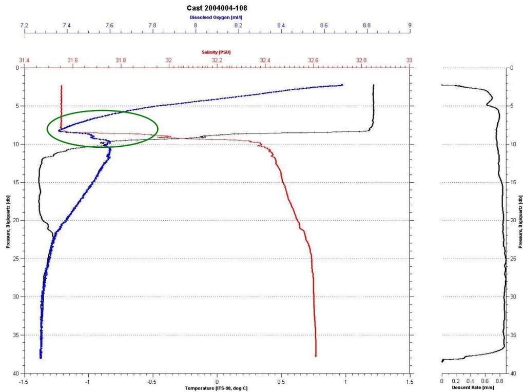
**B 1.** An example of oxygen artefact coinciding with a thermocline (the alignment correction is 10 seconds).
