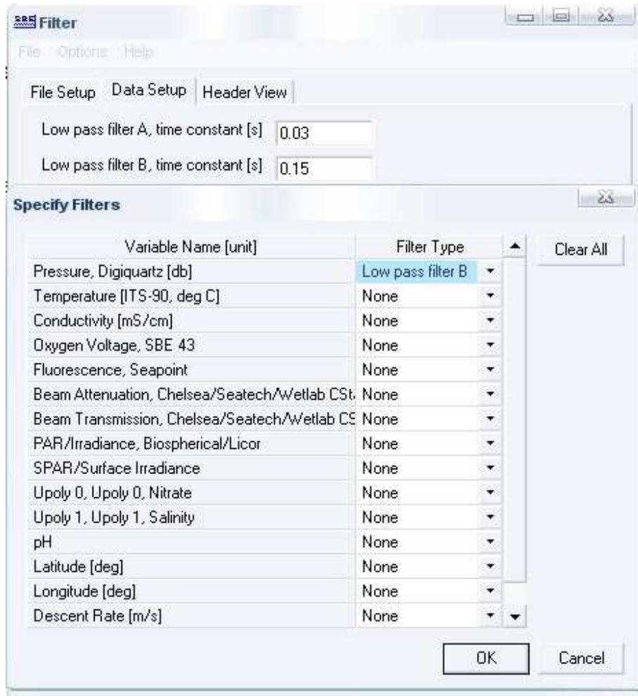
**Figure 5.** The “Filter” module
