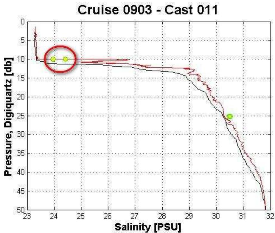
**Figure 26.** Comparison of the salinity difference between CTD and bottles for the cast 011.
