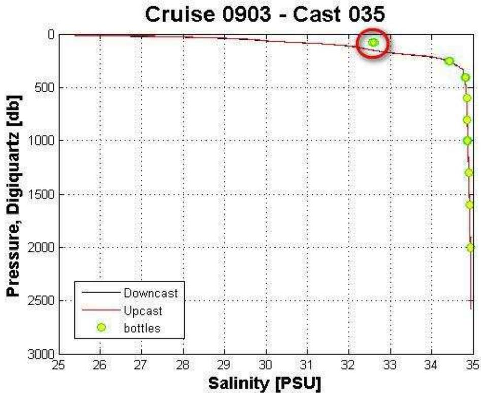
**Figure 27.** Comparison of the salinity difference between CTD and bottles for the cast 035.
