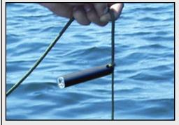
For field deployments, the Minilog 12 TR unit is attached to a cable through a 6 mm [¼"] hole in the non-sensor end.
