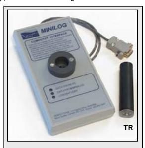
The Minilog 12 is used to collect temperature data for aquatic animal behaviour monitoring purposes.
