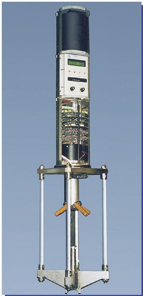
The **CM-04** consists of four piezoelectric transducers and acoustic mirror positioned to measure velocities in two axes, a flux-gate compass unit and a temperature sensor. These, combined with high stability electronics, user-friendly controls and the titanium components, provide for an accurate, stable and durable oceanographic instrument.
