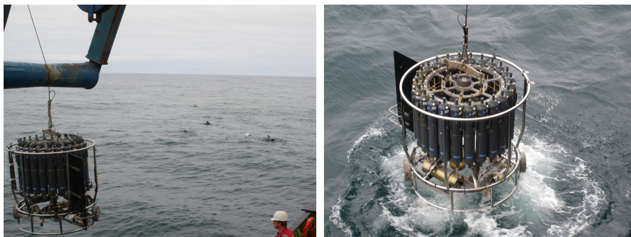
Fig. 4.1 The stainless steel CTD frame with its rosette of 24 20 litre Niskin bottles, and occasional onlookers.
