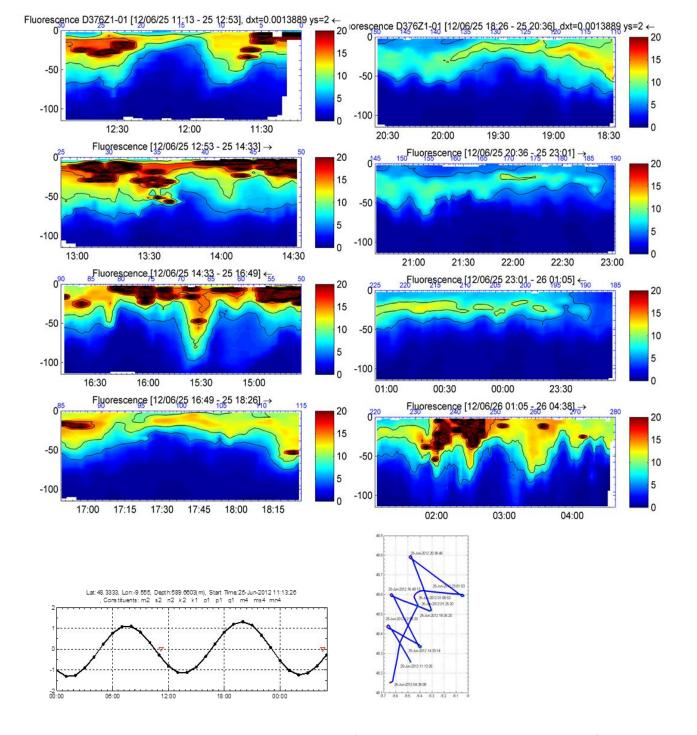
Figure 6.9d. Vertical distributions of fluorescence ( $\mu$ g L<sup>-1</sup>) along the FSI Scanfish Zigzag transects 25<sup>th</sup> - 26<sup>th</sup> June 2012.
