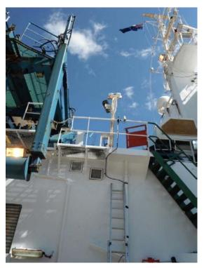
Iridium (satellite phone) and FreeWave (short range wireless data communications with a glider) Antennas, Starboard – Close to CTD winch to the right of the spotlight mounting External antennas allowed short range (<=2km) wireless glider communications and Iridium Satellite phone calls using
