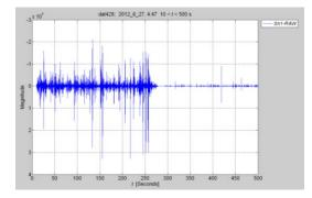
Shear 1 channel - X axis - high and low level signals throughout the data set indicating that the probe is operating correctly.
