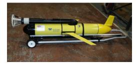
The Unit 175 Turbulence Glider 200m depth capable. The science sensors are a non-pumped Seabird CTD and a specialist micro-Rider turbulence probe
