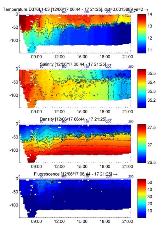
Figure 6.2. Vertical distribution of temperature, salinity, potential density and Fluorescence along the FSI Scanfish transect form Shelf Break to Jones Bank, Leg 1 from SW to NE, 17<sup>th</sup> June 2012.
