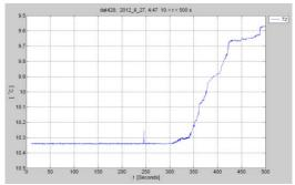
Temperture probe T2 shows rapid measuremnts of water column temperature changes indicating the probe is operating correctly.
