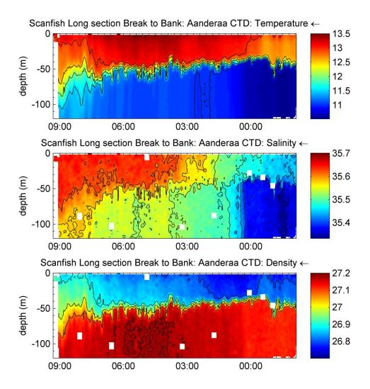
Figure 6.5. Vertical distributions of temperature, salinity, potential density along the AANDERAA Scanfish transect form Jones Bank to Shelf Break, Leg 2 from NE to SW, 17<sup>th</sup> - 18<sup>th</sup> June 2012.
