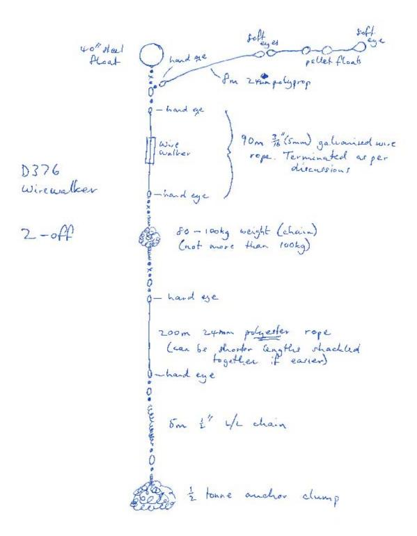
Figure 10.2: Wirewalker mooring diagram
