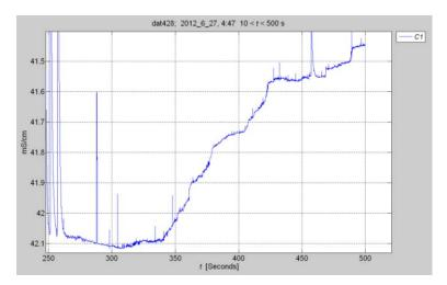
Micro-conductivity measurements demonstrating the probe is still producing rapid measurments in conductivity changes during glider profiling at the end of the deployment. No indication of fouling of the micro-conductivity probes is evident in the recorded data that has been analysed to date
