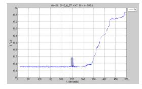
Temperture probe T1 shows rapid measuremnts of water column temperature changes indicating the probe is operating correctly.
