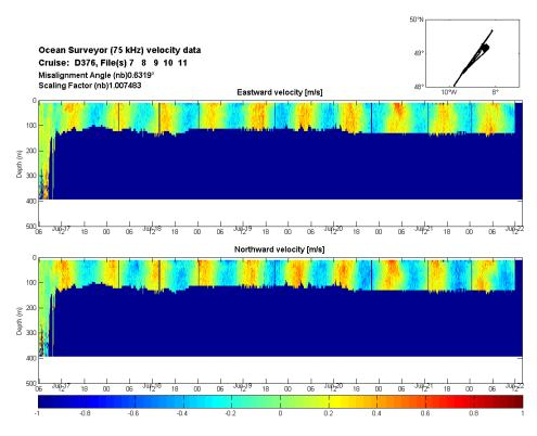
Figure 5.2 Example processed OS75 VMADCP data covering several days and tidal cycles on the shelf
