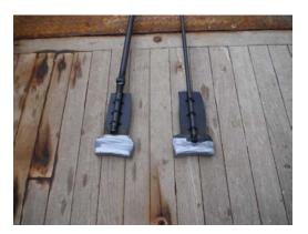
Curved cushioned ends were added to the dual fending off poles. The requirement was to aim for the glider hull fore and aft sections, clear of nose, air bladder cowling, wings and CTD
