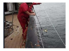
Unit 175 Turbulence Glider alignment for recovery
