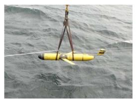
Deployment of unit 051 – Bellamite without a tether for initial dive testing
