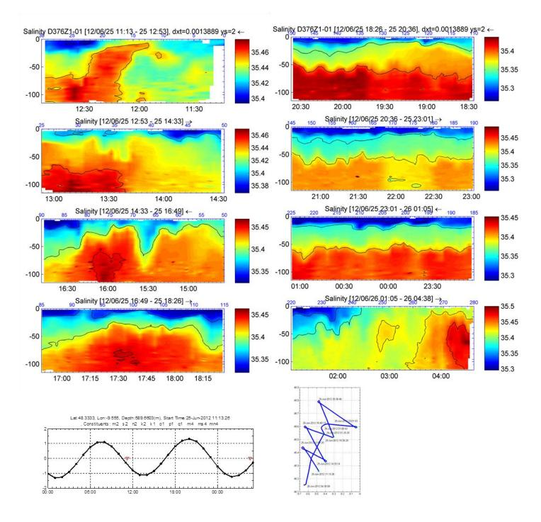
Figure 6.9b. Vertical distributions of salinity along the FSI Scanfish Zigzag transects 25<sup>th</sup> - 26<sup>th</sup> June 2012.
