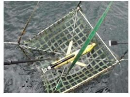
Cushioned fending off poles used for the Unit 175 Turbulence Glider recovery
