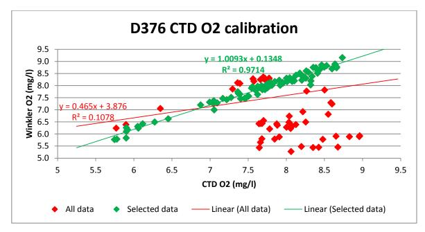
Figure 4.5: CTD  $O_2$  calibration data and equation. Full dataset in red, selected data only in green. Final calibration data in green.
