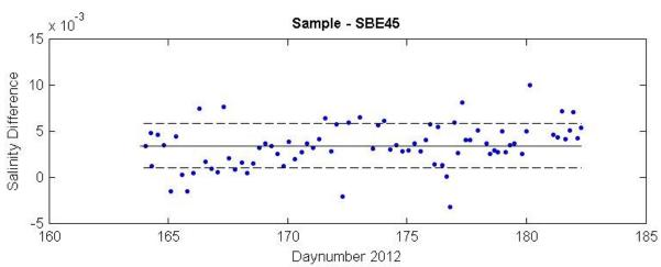
Figure 14.1 Residual salinity (Sample – SBE45). Dashed lines mark 1 standard deviation above and below the mean residual (solid line)
