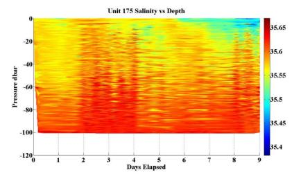
Glider salinity measurements over the 9 day unit 175 turbulence glider deployment Figure 13.12 Glider CTD profiles have been recorded over the full deployment
