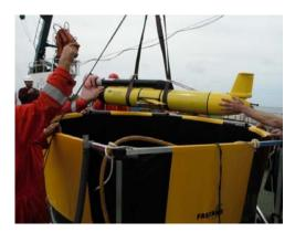
Glider release arrangement testing
