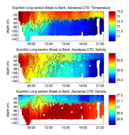
Figure 6.4. Vertical distributions of temperature, salinity, potential density along the AANDERAA Scanfish transect form Shelf Break to Jones Bank, Leg 1 from SW to NE, 17<sup>th</sup> June 2012.
