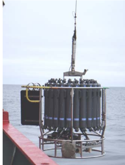
Figure 1.1-1: CTD being deployed from the mid-ship gantry.
