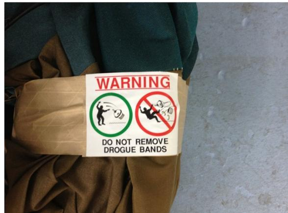
There are no pre-deployment checks to perform or settings to configure. Do not unravel the tether from the cardboard spool. Do not remove the drogue bands. (Both the tether spool and the drogue bands are held in place with water soluble tape that will release once in the water. Unraveling the tether or removing the drogue bands can be dangerous for the operator upon deployment.
