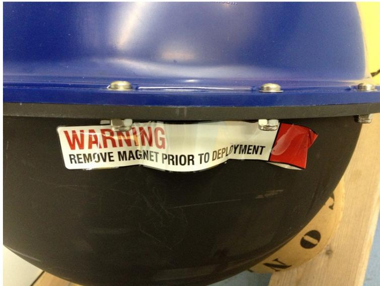
The SVP is designed for a maximum free fall height of 10 m. The SVP and drogue should be held and dropped together.
