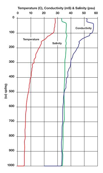
The Expendable Conductivity/ Temperature/Depth (XCTD) Profiling System is an accurate and cost-effective means to collect salinity profiles while underway. The system consists of the Digital XCTD probe, developed by the Tsurumi Seiki (TSK) Co. Ltd. Of Yokohama, Japan and Lockheed Martin's representative and licensed manufacturer of XBTs in Japan. Three models of XCTD are available for different depths and ship speeds.
