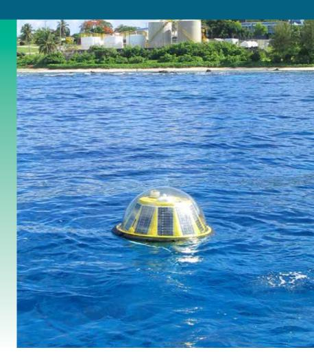
The TRIAXYS™ Directional Wave Buoy uses the TRIAXYS™ Next Wave II Sensor for continuous wave sampling and accurate wave data.
