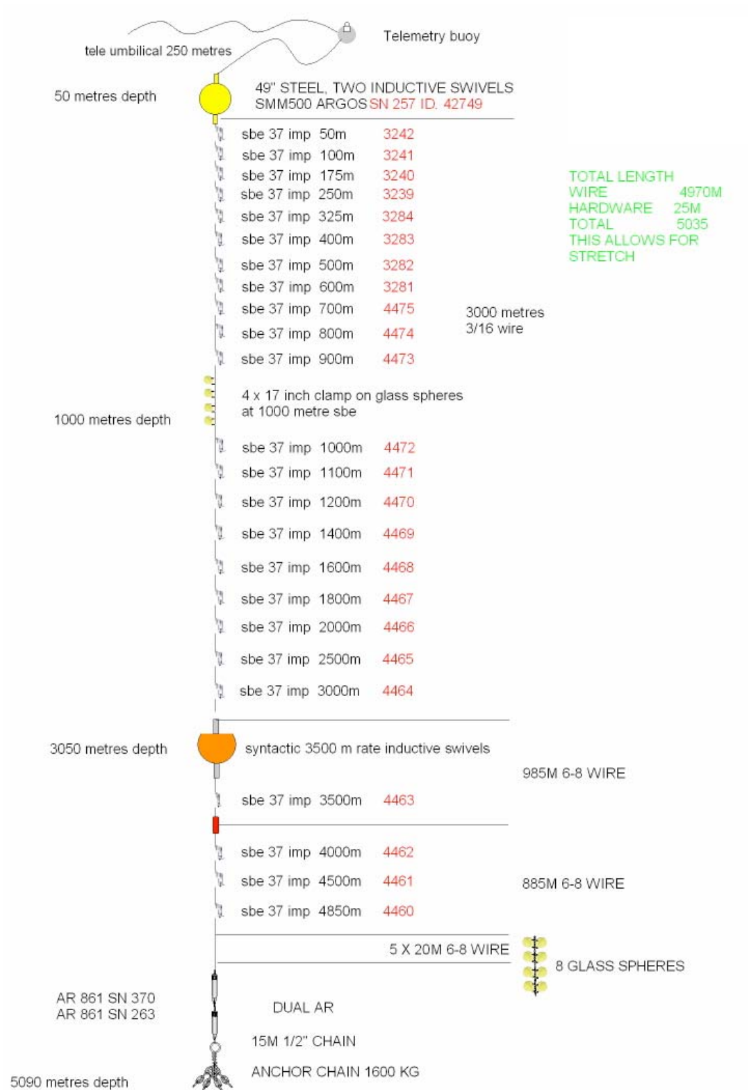
Figure A.6: Mooring diagram of EB1_3_200561 as deployed on CD177
