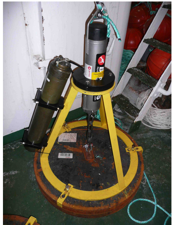
Figure 5: Tripod base of mooring with anchor weight, aluminium case for BPR and acoustic release.
