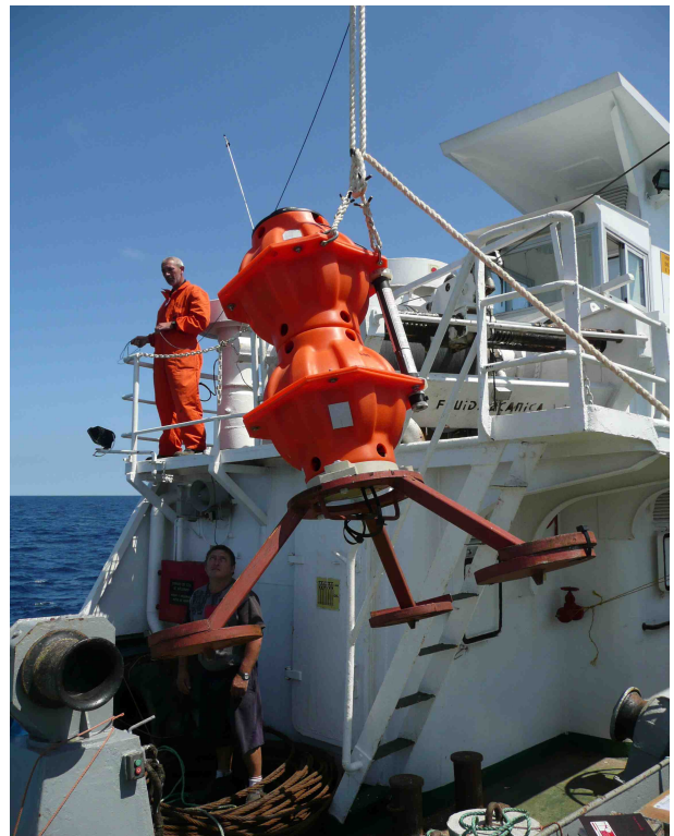
Figure 3: BPR lander "Mareografo 2" during deployment.
