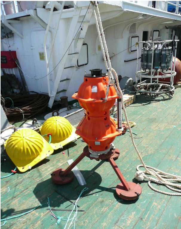
Figure 2: BPR lander "Mareografo 2" on aft deck immediately before deployment. Note the Novatec beacon on the right hand side.
