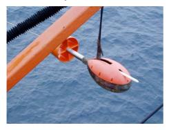
During D285 a total of 210 surface samples were collected during the cruise. Water was pumped up from the clean fish (Fig. 7.1) at a depth of ~6m and into the clean container where it was withdrawn at the manifold either un-filtered or through a 0.2  $\mu$ m filter cartridge.
