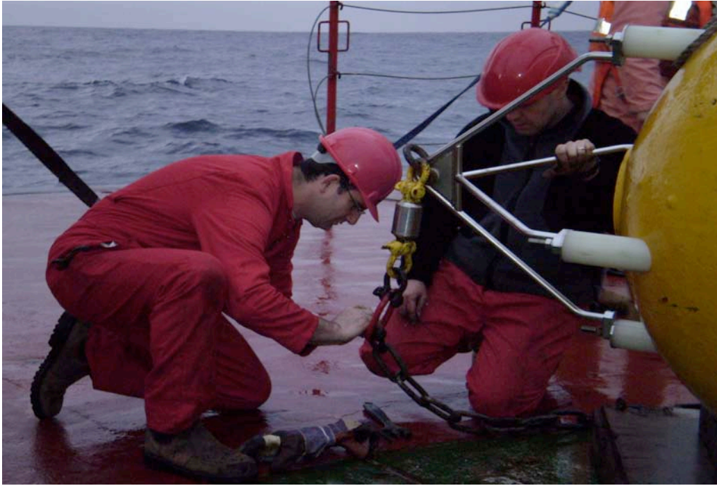
Figure 9: Final preparation of the sub-surface syntactic sphere housing the LR-ADCP.
