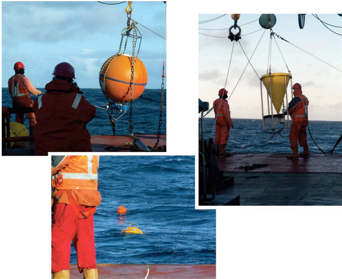
Figure 2: Deployment of the SC-ADCP (left and bottom) and sediment trap (right) at STC.
