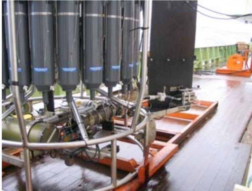
Figure 35: Detail of the CTD frame and rosette sampler system. The primary CTD sensors are attached to the bottom of the vane on the right. The secondary sensors are strapped to the top of the right hand horizontal cylinder beneath the bottles.
