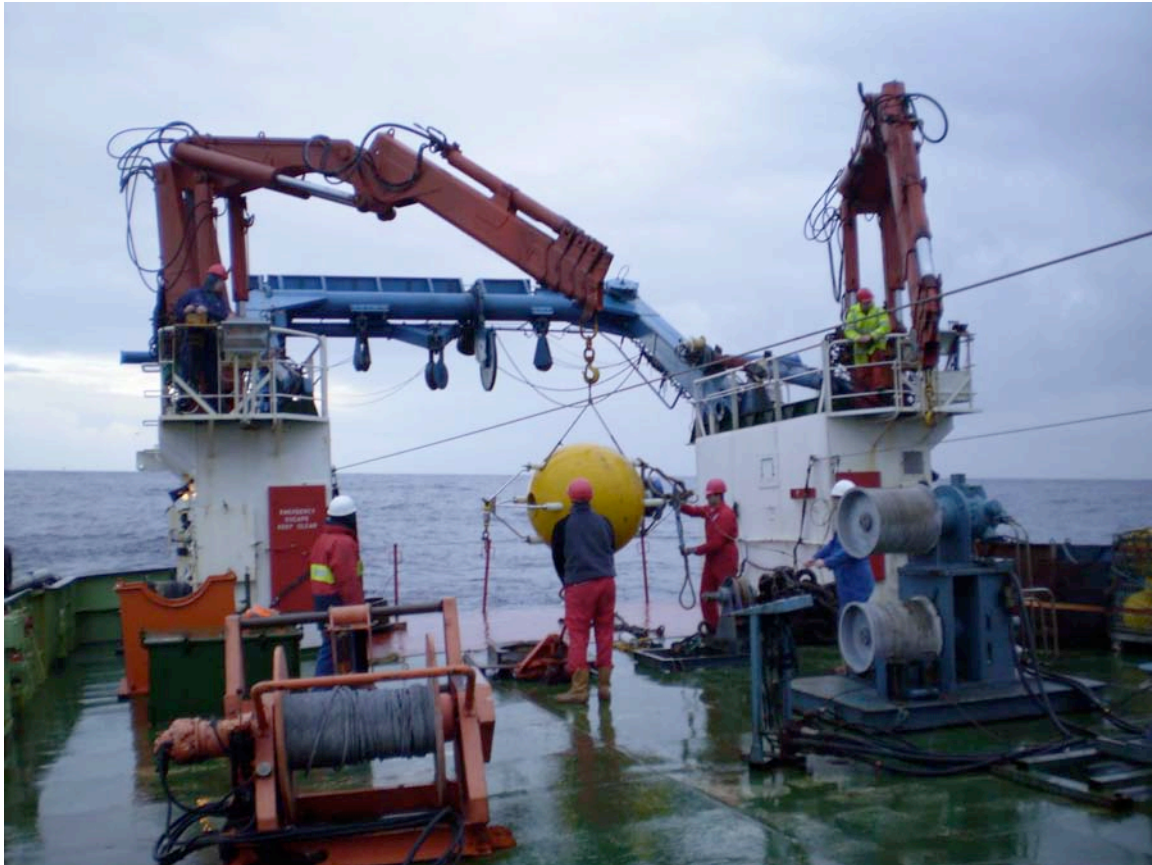
Figure 8: Mooring components being moved into place prior to deployment of the mooring over the stern.
