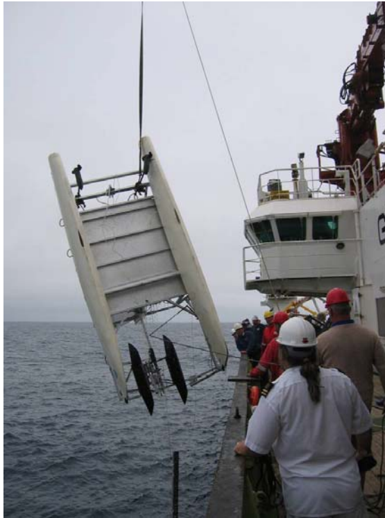
Figure 69. Ventral view of the remote controlled catamaran and skimmer holding the glass drum (between the floaters).
