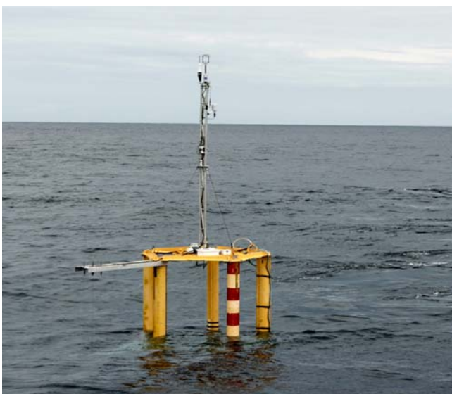
Figure 21. Photo of ASIS2 being deployed from RSS Discovery. Once deployed, ASIS becomes vertical, with the mean waterline at the middle red stripe. Each strip is ~30cm wide. Sensors visible on ASIS are: A: URI package; B: Data acquisition systems, including motion package, and batteries; C: SAMI package; D: SST; E: Dopbeam; F: SAMI; G: Wave-staff array (outrigger visible); H: Air temperature, humidity; I: Sonic anemometer, Licor.
