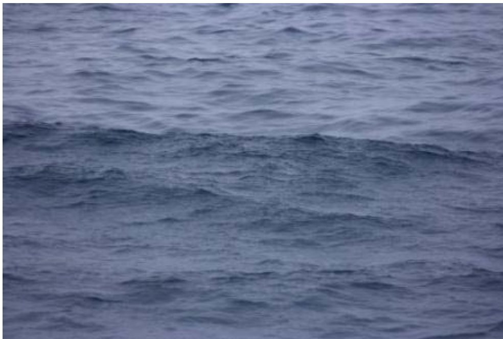
Frontispiece: An artificial surfactant patch edge showing clear suppression of capillary waves (Robin Pascal).
