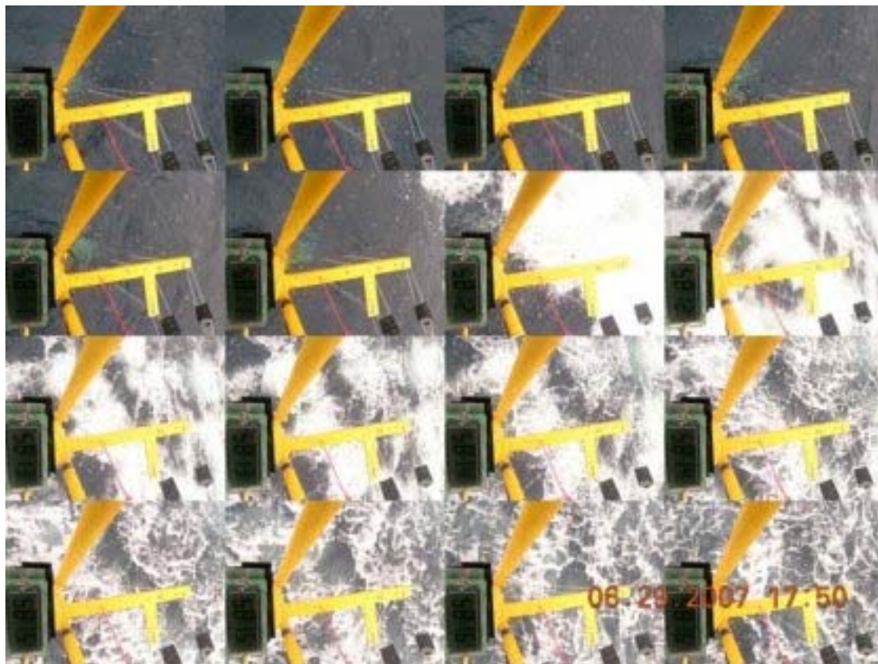
Figure 56. A run of 16 images captured by the Nikon 5400 stills camera on the second deployment. A breaking wave and the white froth it leaves in its wake can clearly be seen passing through the buoy.
