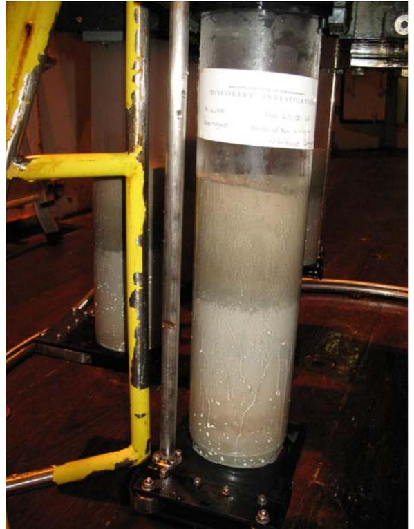
*Figure 20: A core from taken showing layering. Top is soupy material, then a sandy layer, followed by a heavier mud.*
