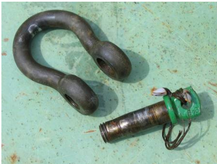
Figure 6. Photograph showing erosion of threads in main shackle holding instrument frame to buoy
