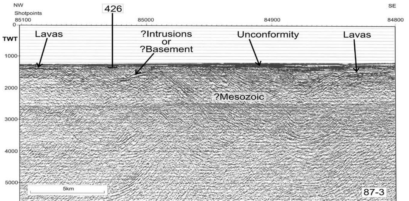
Figure 13. Seismic line through site 426. For location see Figure 1.
