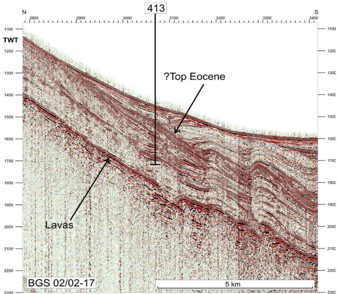
Figure 9. Seismic line through site 413. For location see Figure 1.
