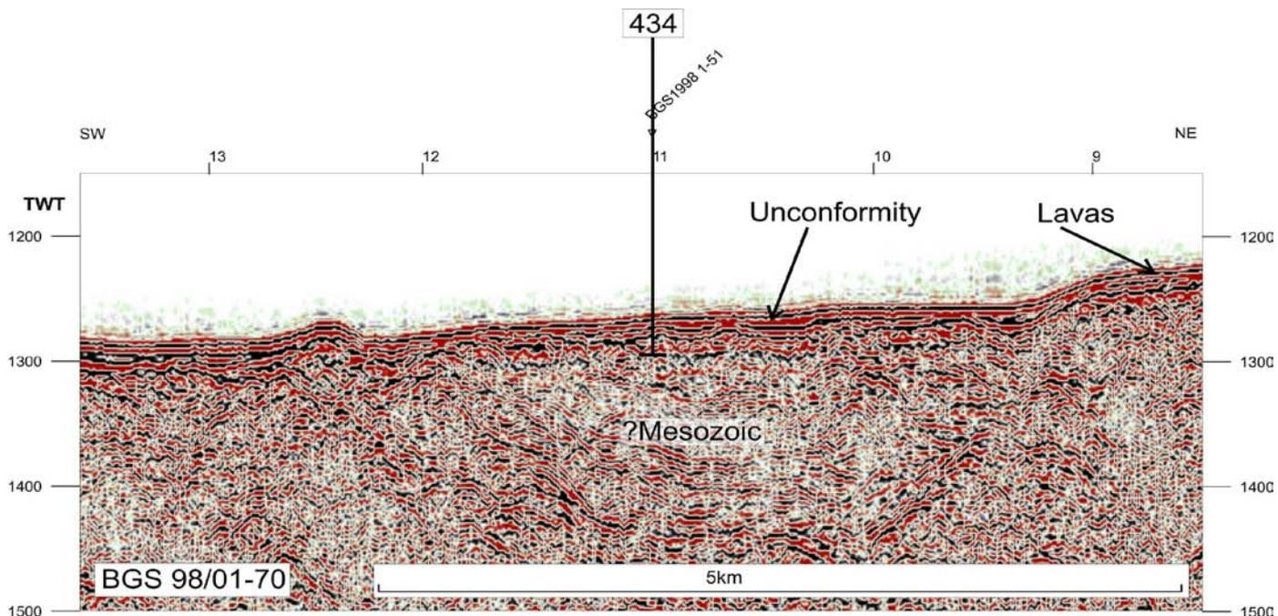
Figure 17. Seismic line through site 434. For location see Figure 1.
