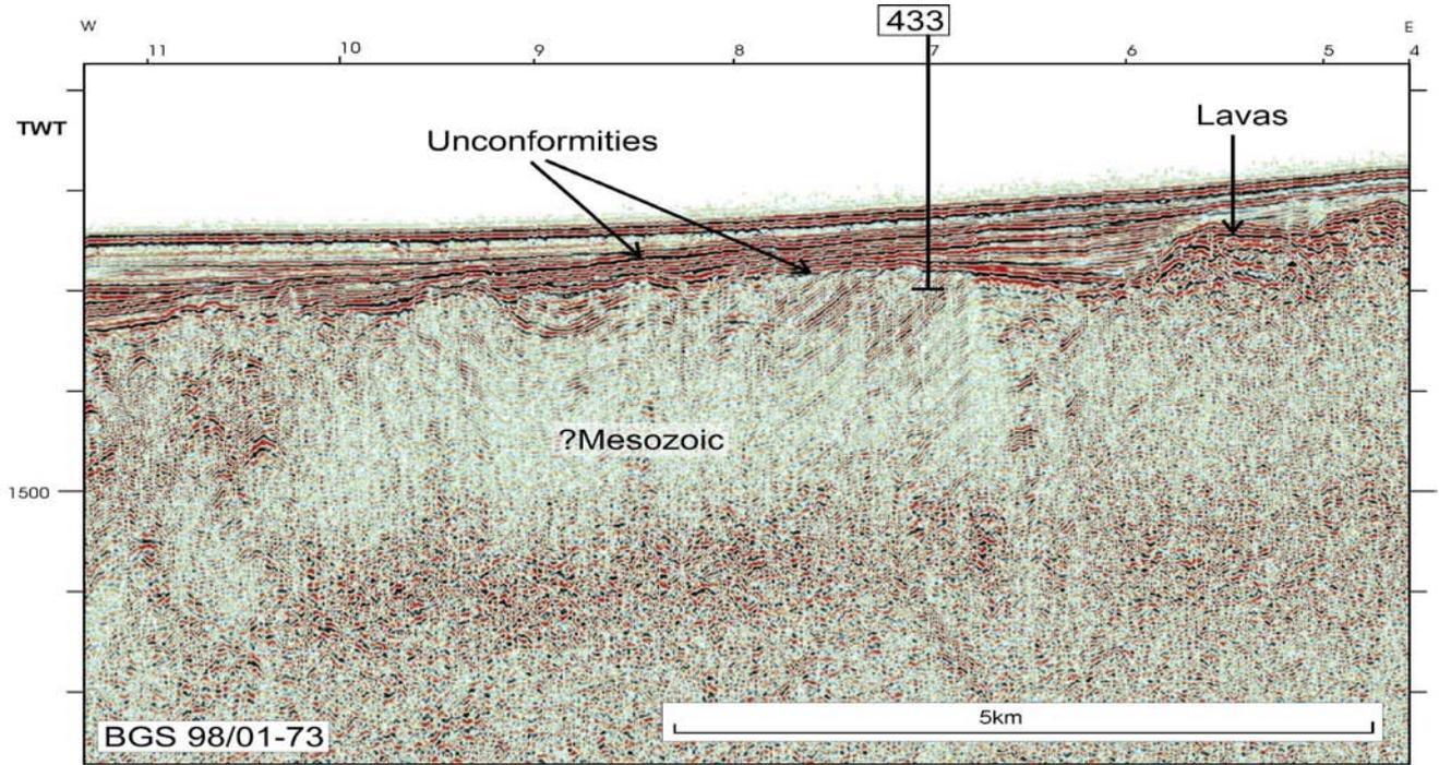
Figure 16. Seismic line through site 433. For location see Figure 1.
