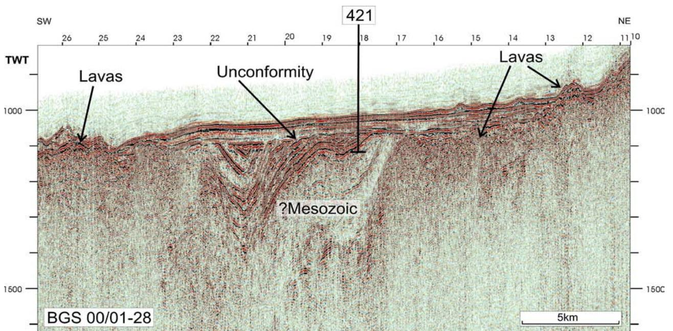
Figure 11. Seismic line through site 421. For location see Figure 1.
