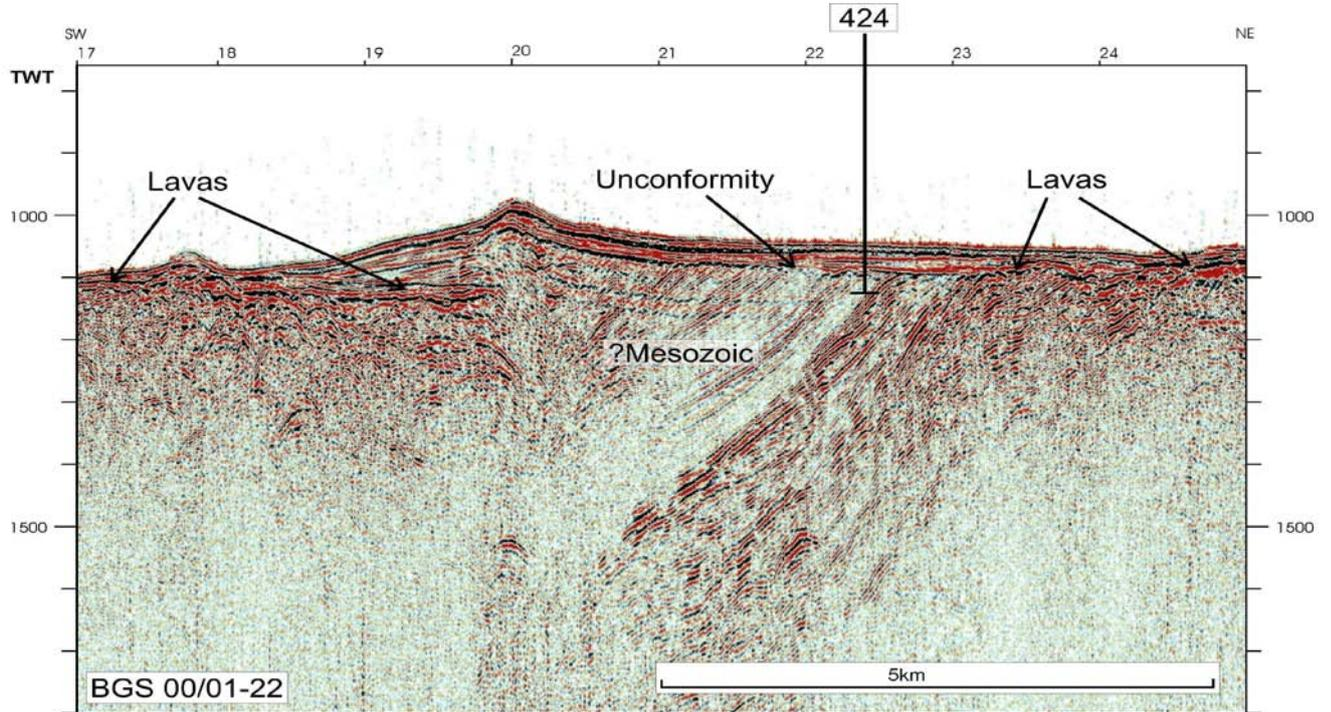
Figure 12. Seismic line through site 424. For location see Figure 1.
