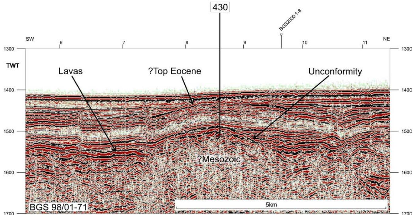
Figure 15. Seismic line through site 430. For location see Figure 1.
