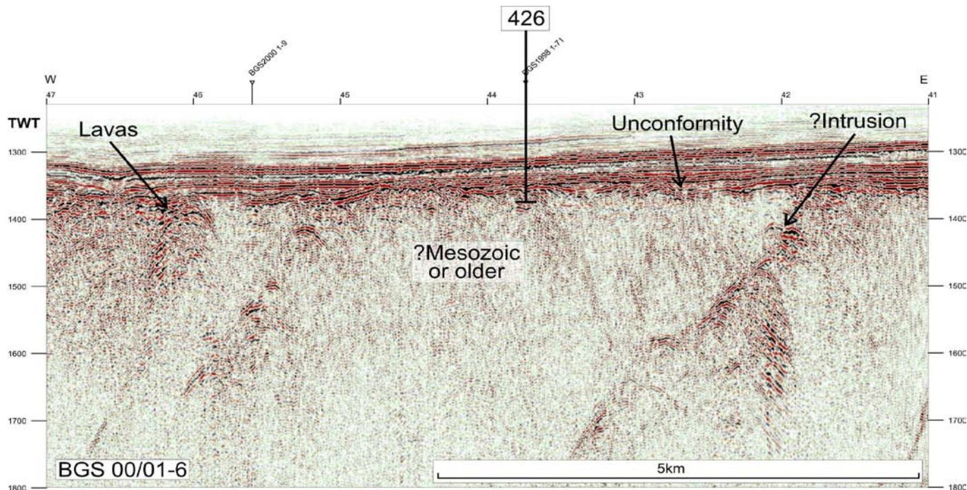
Figure 14. High-resolution seismic line across site 426. The borehole will penetrate ?Mesozoic (or older?) sediments below the base Cenozoic unconformity in the large basalt window. See also line 87-3 (Figure 13) for more regional profile.
