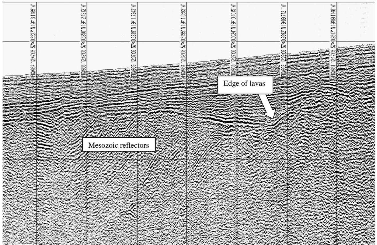
Figure 31. Example of site survey line collected using sparker equipment.
