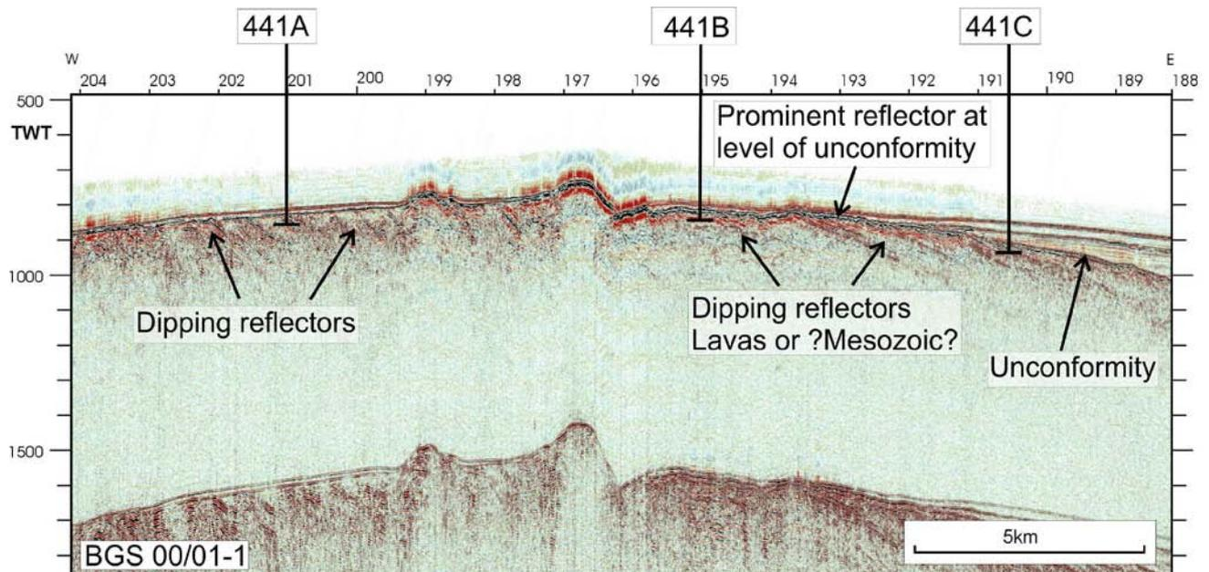
Figure 18. Seismic line through site 441. For location see Figure 1.
