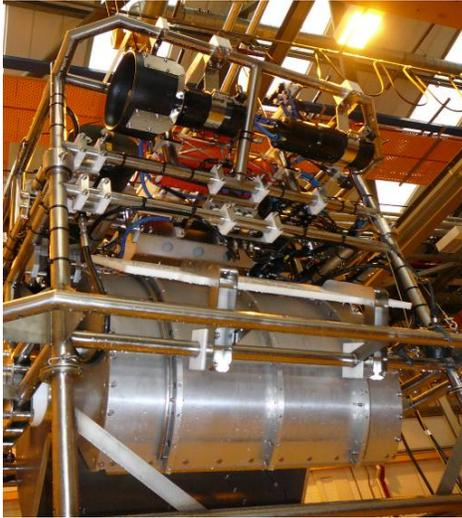
HyBIS has a command module for power, lights, and telemetry, and a swappable tool module for sampling. The command module has twin colour cameras and over 1000W of lights - all rated to 6000m. The command module also has hydraulic power packs, 140Bar water pump and electric thrusters producing 100 kg of thrust. The sampling module currently comprises a 0.3 cubic meter clam-shell grab.
