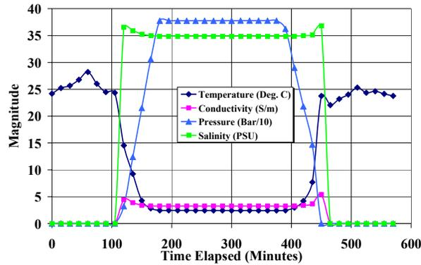
**Fig. 5 – Recorded Seabird Microcat CTD Data during the MYRTLE Deployment and Recovery**
