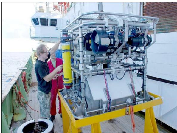
The HyBIS vehicle mounted on its deck stand, on the starboard deck of the RRS Discovery. Dr Bramley Murton (shorts) and Veit Hunnerbach (red boiler suit) mounting the U SBL beacon (yellow tube) on to the vehicle.
