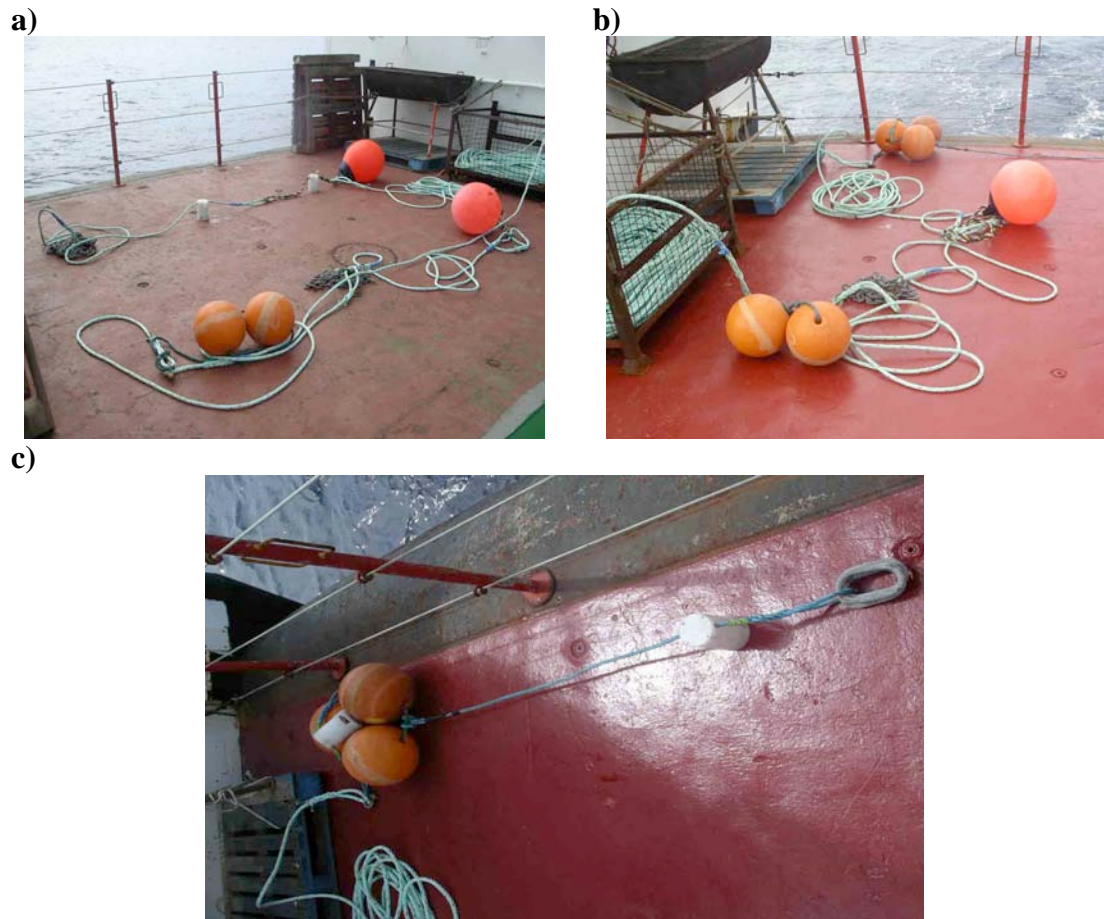
Figure 66: Photographs of showing the development of the near surface salinity buoy system showing a) 2 sensors mounted on initial 5m long chain-weighted rope; b) and c) showing later shallower, lighter system.
