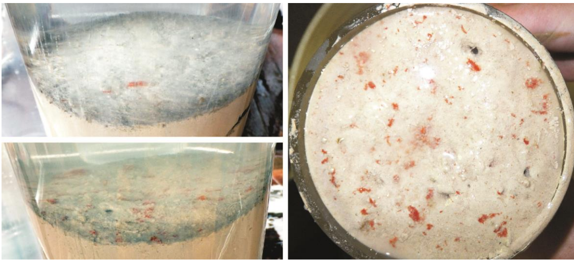
Fig. 3.3.16. 'Red fluff' noted on core tops from site E1, core tube internal diameter 10cm (stn D377-010).
