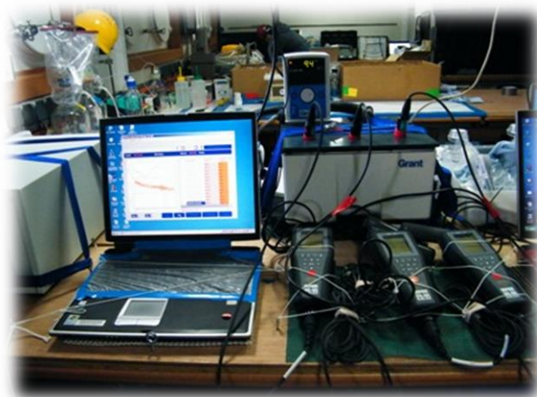
Figure 15. YSI ProODO optodes deployment and the water bath used.
