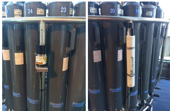
Figure 11. Wirewalker sensors strapped to the Stainless Steel CTD for calibration dip
