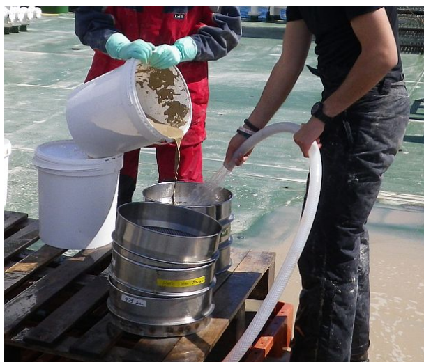
Fig. 17.4 Elutriation from 20 litre collecting bucket into 4 mm, 0.5mm and 0.42 mm sieves.
