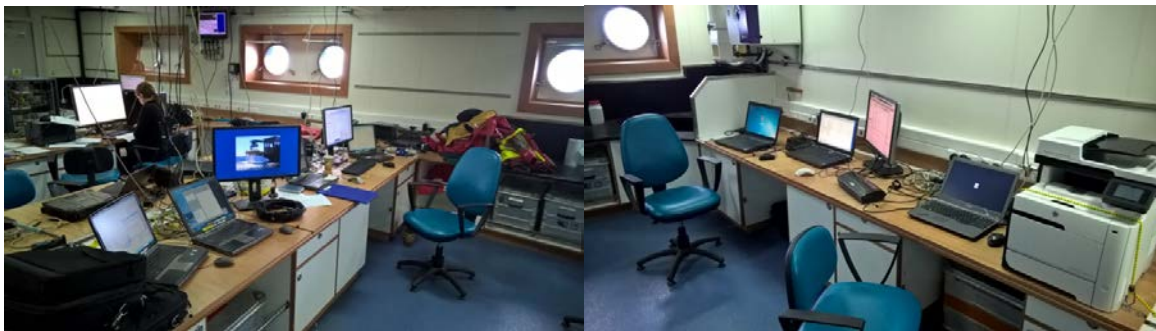
Figure 19.9. Main lab area forward, port side. Left image station in order from left: tracking and telemetry, sonar control, mission management. Right image in order left to right: 2x data processing then Iridium communications.
