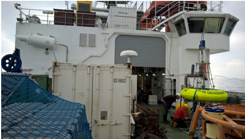
Figure 19.8. Container aft deck port side forward. Gantry port side under the A frame. Iridium Antenna on top
