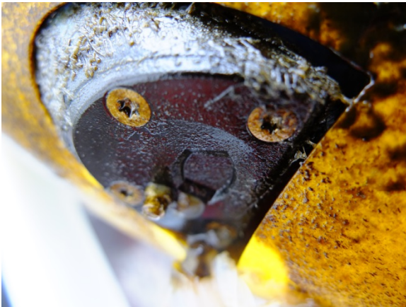
Figure 20.2. The Seaglider showed much less fouling as expected, with the PAR sensor clean and little or no slime over the other sensors and upper surface, and with only 2 or 3 tiny barnacles on board. The optical sensors were unfouled.
