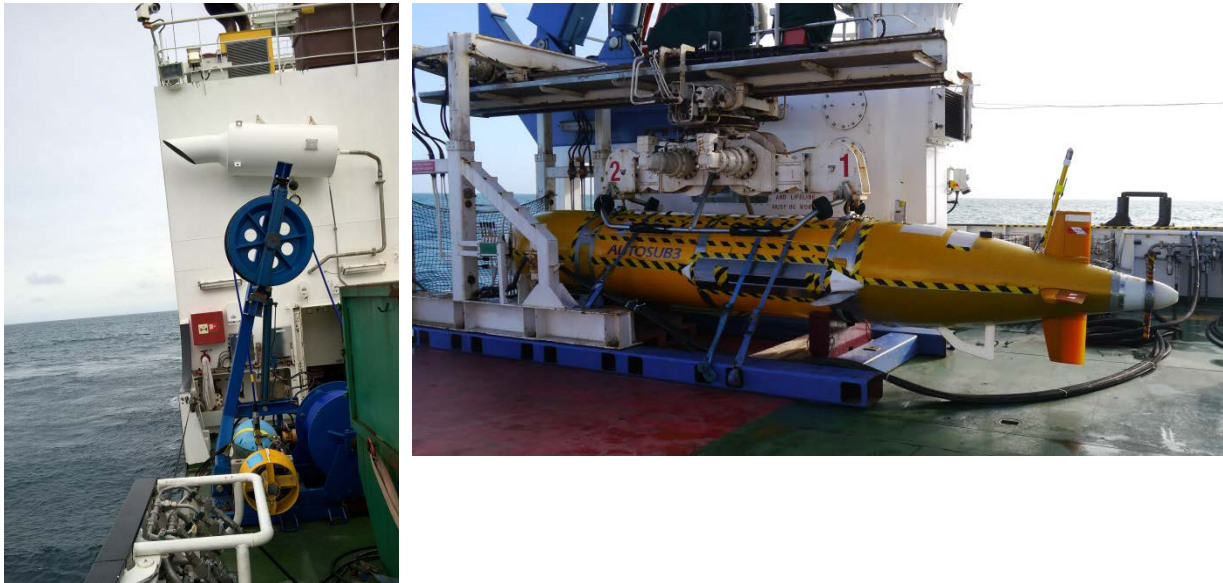
Figure 19.7. Launch, Relocation and Recovery as per all SSB cruises. Left: Acoustic Tracking and Telemetry Fish and PES winch. Right: Launch and Recovery System.
