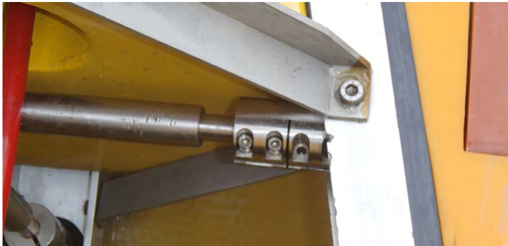
Figure 19.15. Port side coupling outer portion was slipping during M463 (note the bolts removed in this picture were in place during the deployment)
