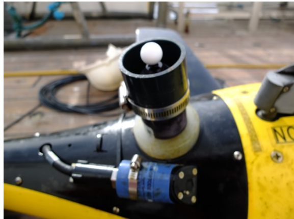
Figure 20.2. The Seaglider showed much less fouling as expected, with the PAR sensor clean and little or no slime over the other sensors and upper surface, and with only 2 or 3 tiny barnacles on board. The optical sensors were unfouled.
