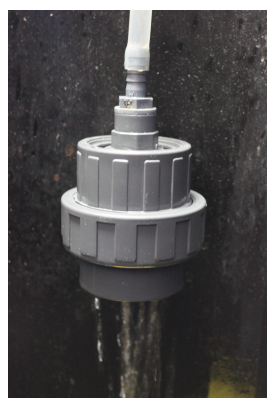
Figure 16.1. Microplastic filtration of ships underway water system. A 80µm mesh filter is sealed within the grey PVC housing to avoid filter contamination, water delivered via the clear silicone tubing and discharged into ships sink.
