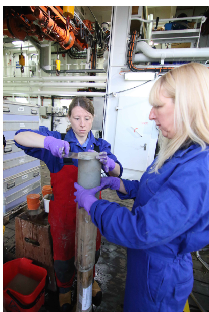
Figure 16.4. Sediment core on the wooden extruder, cores are slicing using a stainless steel cutter into depth horizons.
