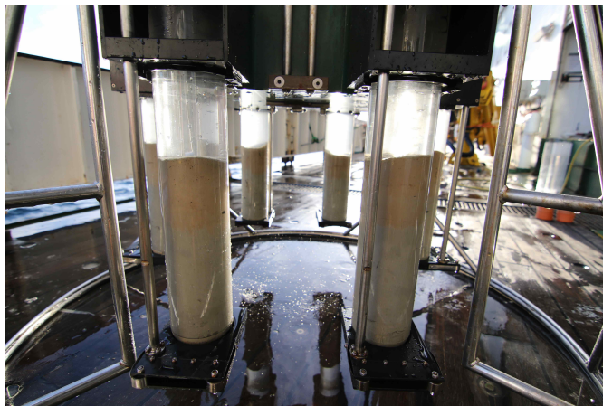
Figure 16.3. The six core tubes filled with sediment, typical sediment depths were between 27 - 30 cm, with 30 – 33 cm of supernatant water.
