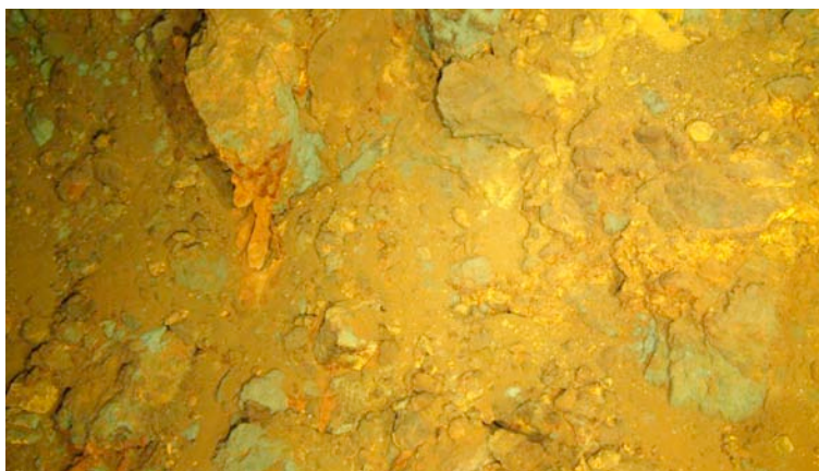
Figure 36. HD still image from HyBIS showing iron and copper mineralisation.
