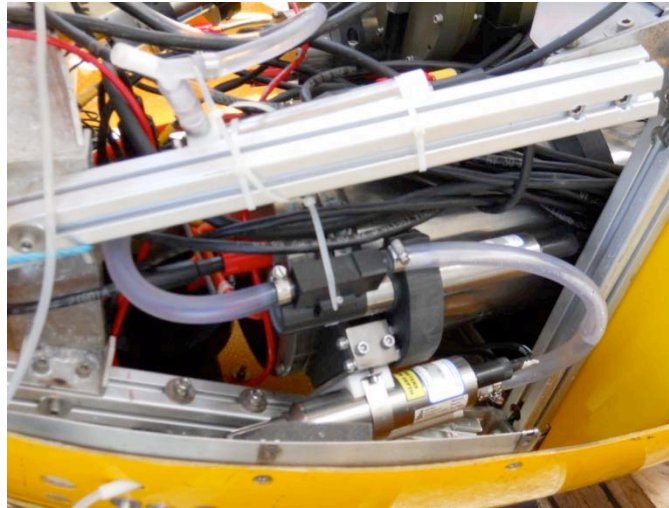
Figure 11. Port CT (mounted below the panel split line) and Oxygen sensor uppermost
