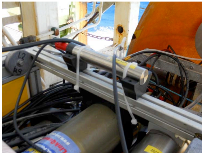
Figure 12. Magnetometer mounted on top of nose frame, avoiding magnetic materials where possible
