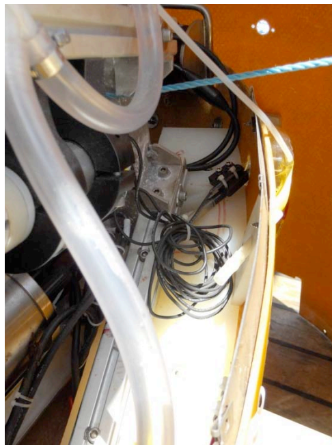
Figure 15. Eh sensor on starboard side protruding through panel
