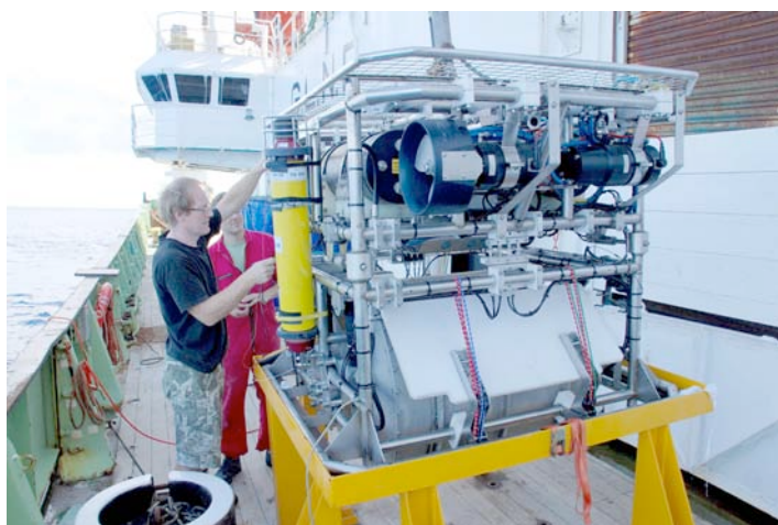
Figure 24. HyBIS in its deck frame being prepared for a deployment by Veit Huehnerbach (red boiler suit) and Bramley Murton. The yellow cylinder is the USBL subsea navigation beacon.
