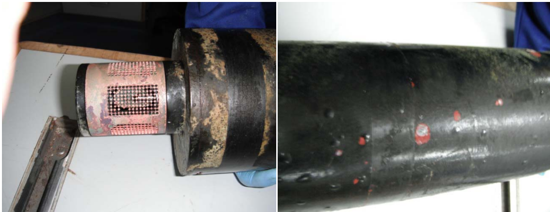
Fig. 21 Damage to copper sensor guard. Fig. 22 Deterioration of pressure case coating.
