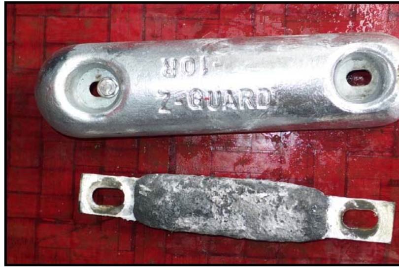
Fig. 6 Sensor frame anodes before and after deployment.
