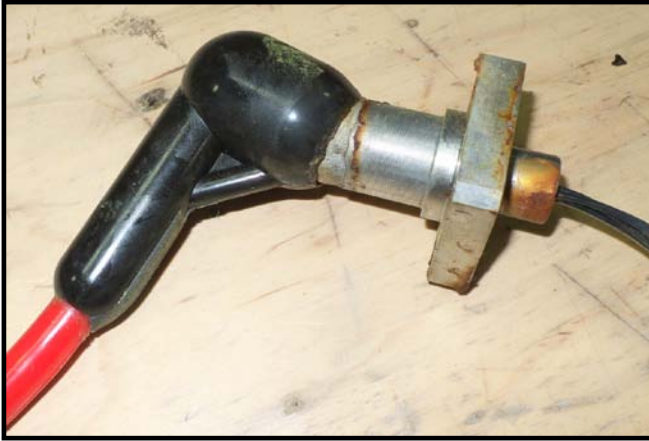
Fig. 8 Penetrator 6 showing moulding separation from stainless steel bulkhead.
