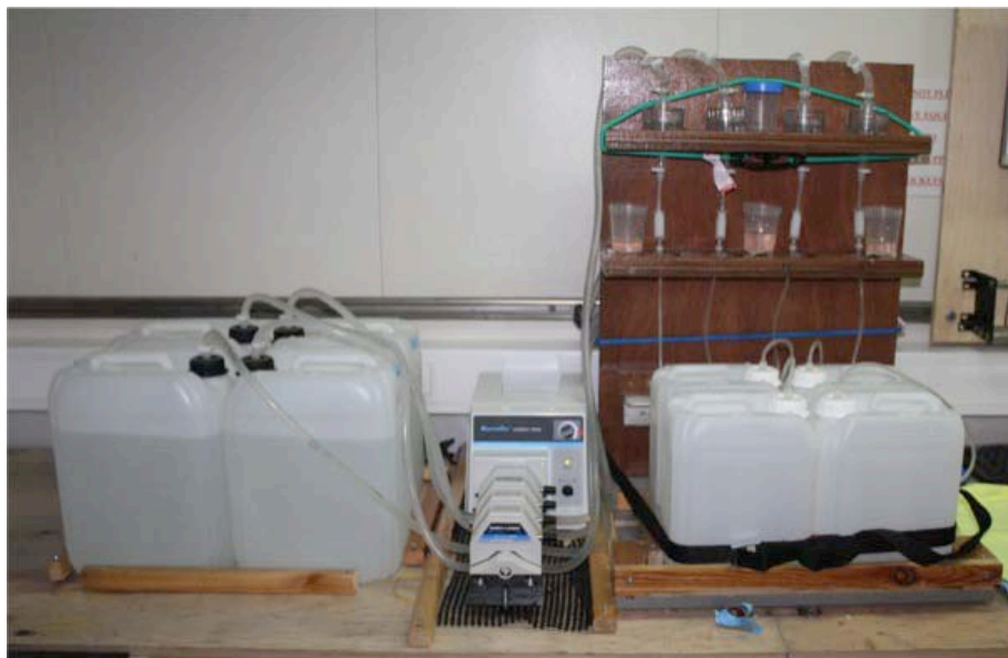
Fig. 38 Two-stage filtration system set up with four samples being processed at the same time.
