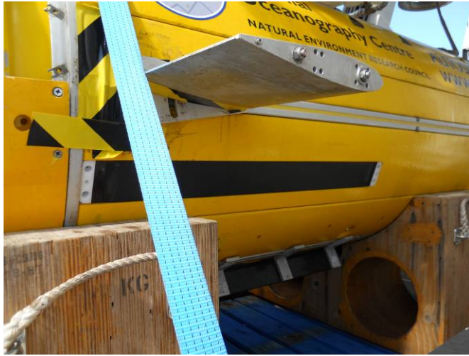
Photo 4. Edgetech Side Scan inset into the centre buoyancy blocks just below the winglets
