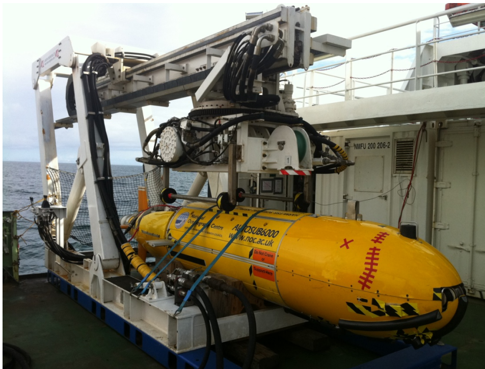
Photo7. The Autosub6000 MKII L&R system installed on the aft deck of the RRS James Cook. The red tape (rather comically) showing the position of some top panel damage due to ship collision on the last recovery
