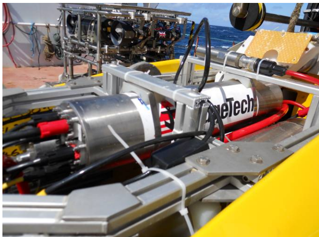
Photo 3. Edgetech electronics mounted in the tail
