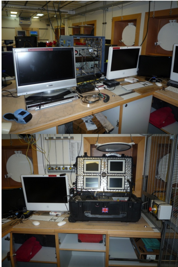
Figure 5.2. left to right, top to bottom: Lab setup showing video screen and logging system arrangements for HyBIS and its main control box.
