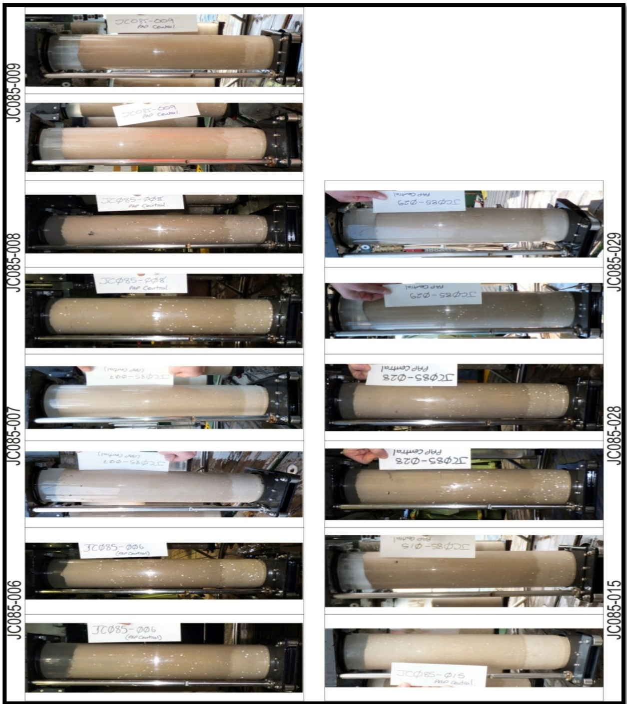
Figure 33: Example Core Profile Photographs from PAP Central Megacorer Deployments during JC085. (scale: core tubes have an internal diameter of 100mm; the white card in view has a length of 176mm).
