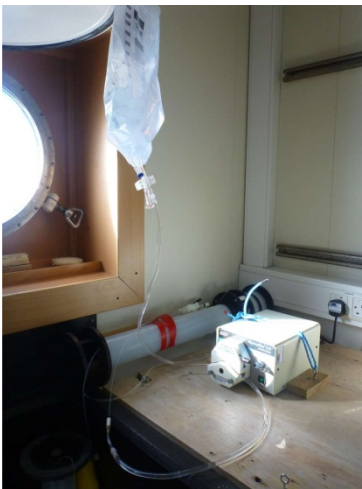
Figure 11: Osmotic sampler preparation A) Filling the sampling tube with MQ water; B) Osmotic Pump; C) Sampler on the frame
