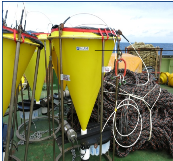
Figure 29: Trap D, inverted and using hyposaline STP, showing the 'this way up' labels to identify it for deployment.
