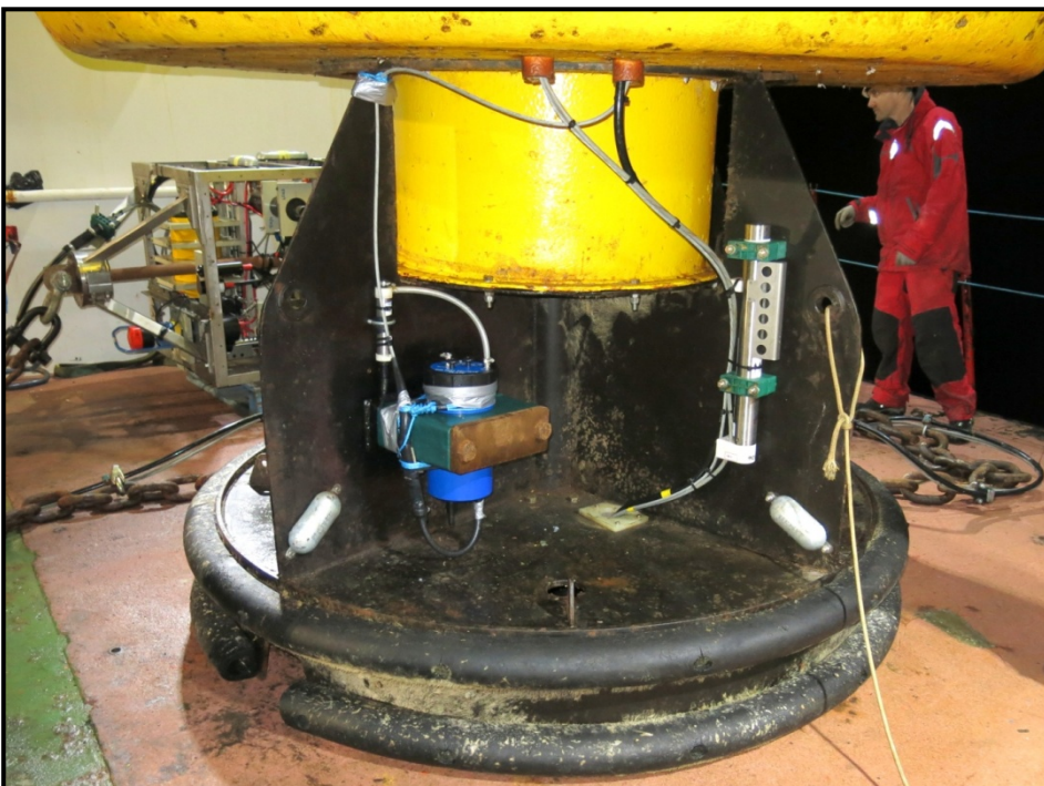
Figure17:5 Pro-Oceanus CO2-Pro and Seabird MicroCAT Sensors Fitted to Buoy Keel
