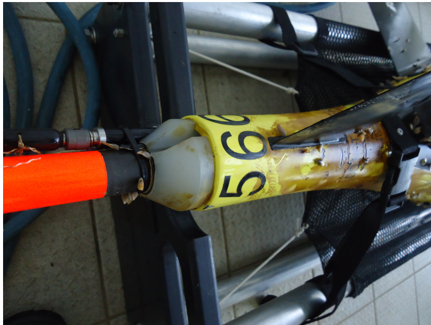
Figure 7: Goose barnacles and algae on Seaglider 566.
