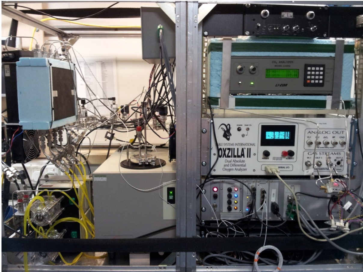
Figure 24: Photograph of the drying unit (left rack) and the measurement unit (right rack). Calibration procedures
