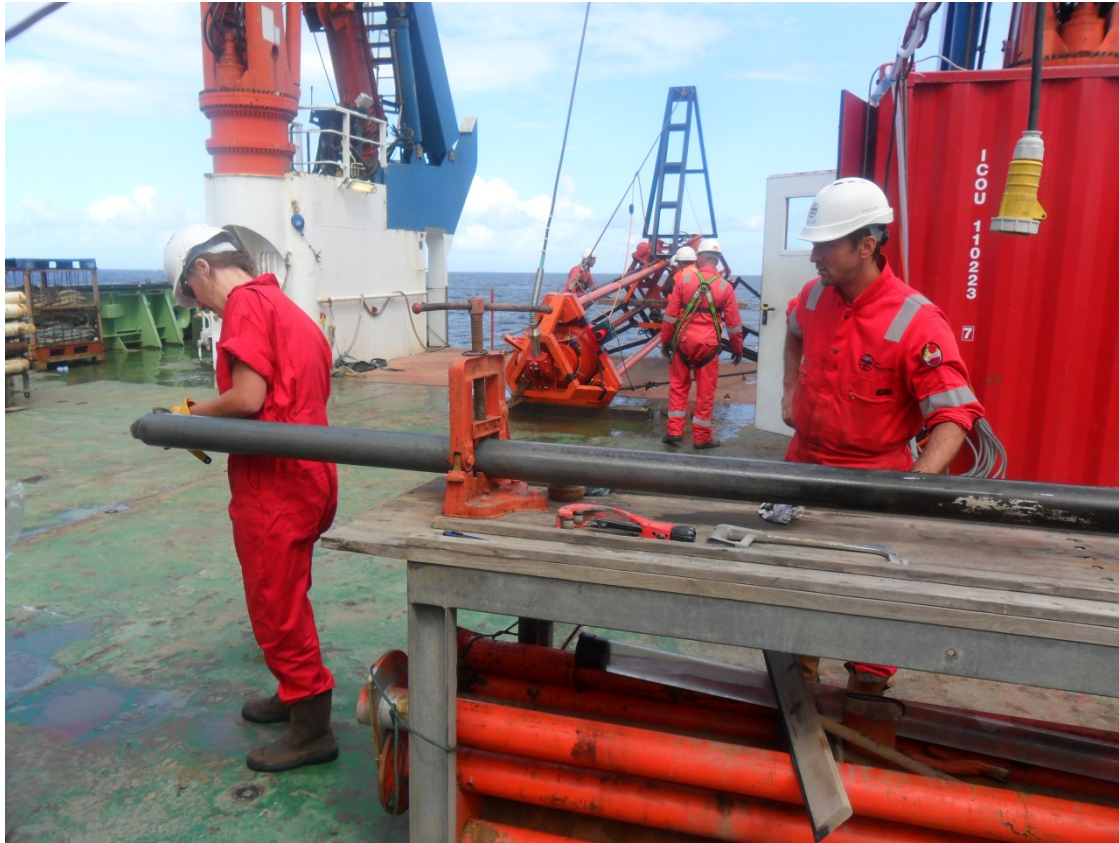
Figure 9. The aft deck with the BGS vibrocore bench and vibrocorer in the background.
