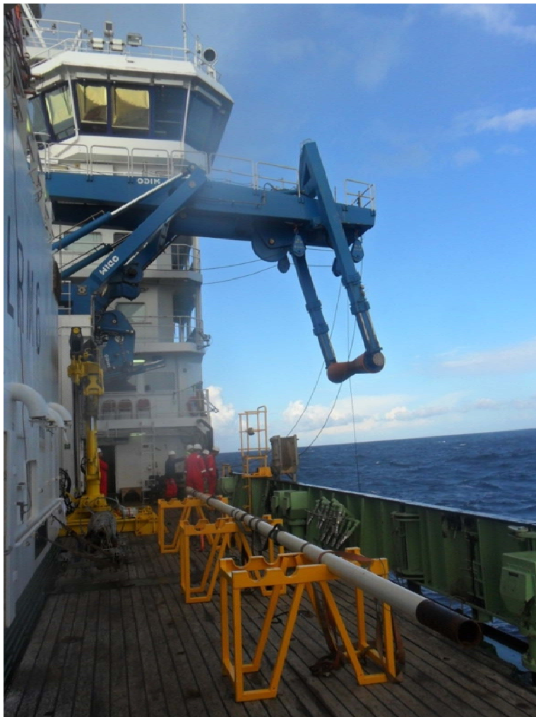
Figure 11. Recovery of piston corer, Malin Sea.
