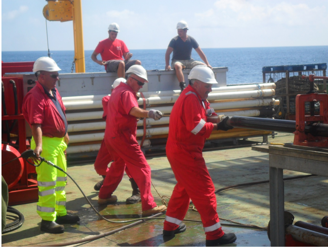
Figure 8. Removing the vibrocore from the core barrel.
