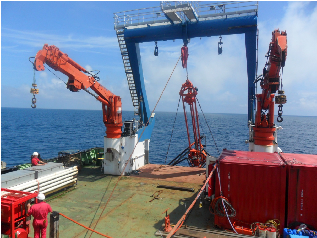
Deployment of the BGS vibrocorer in the Celtic Sea, July 22 nd , 2014
