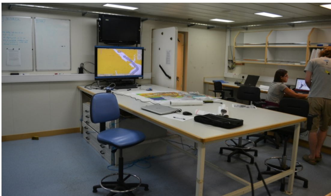
Figure 8. TV screen used by Olex to display current position and planned survey tracks
