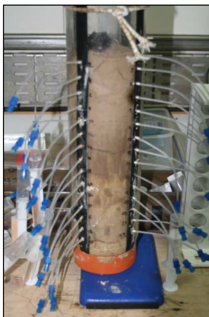
Figure 45. Porewater extraction in Mega Core sample using Rhizons.
