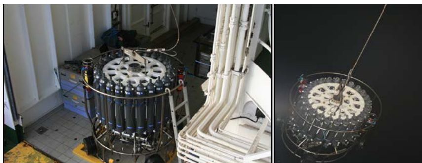
Figure 42. Niskin bottles mounted into the CTD frame before and during deployment.
