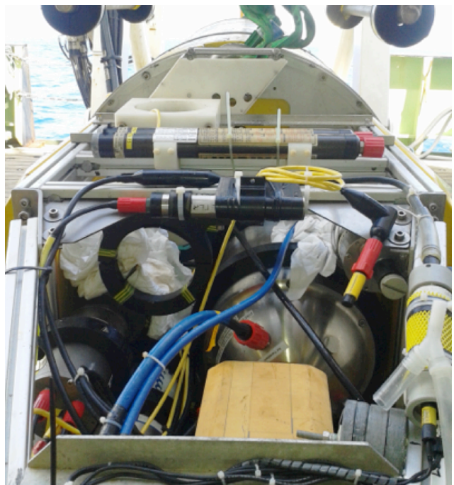
Figure 54: Magnetometer mounted athwartships in Autosub's nose, with red connector on left, attached to the frame, middle-top.
