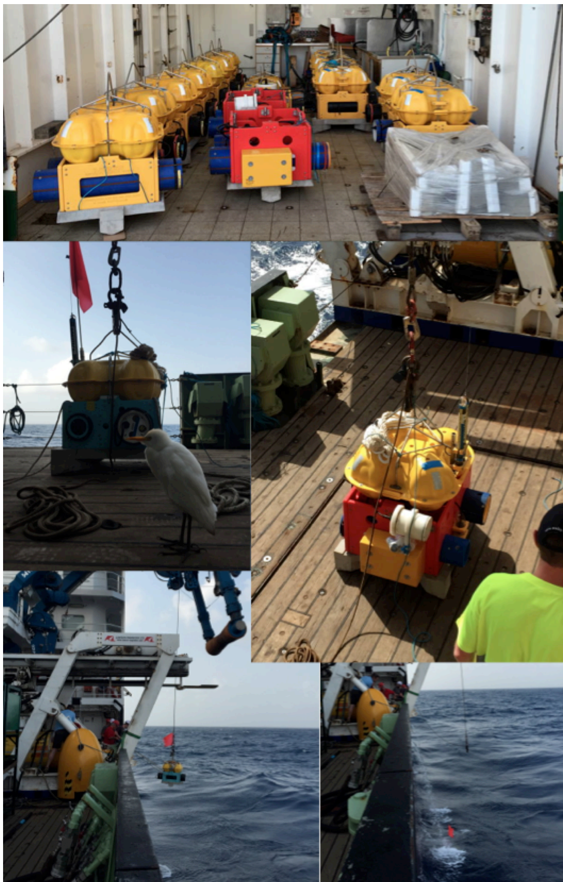
Figure 9: Range of 58 ocean-bottom seismographs deployed during JC132. Top: standard platforms amassed in the water bottle annex ready for deployment. Left middle: standard OBS ready to be deployed over the starboard side. Right middle: broadband test platform variant ready for deployment. Bottom: the last deployment of the cruise.
