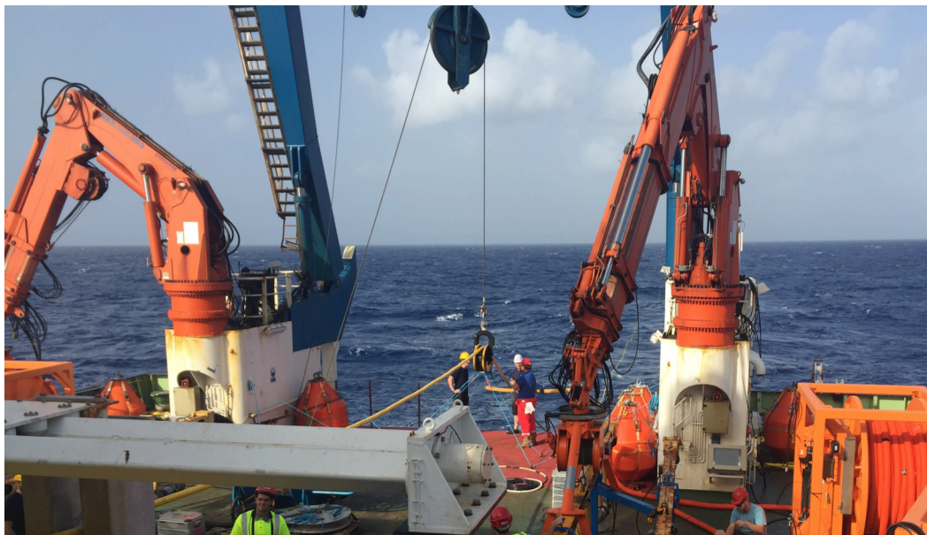
Figure 22: Multichannel seismic streamer during deployment. The yellow Sercel Sentinel streamer is towed from the winch drum (foreground) astern over a fairlead suspended from the stern A-frame (centre of shot). Once deployed, the fairlead is raised to prevent streamer chaffing over the stern rails as the stern of the vessel heaves with the motion of the sea.
