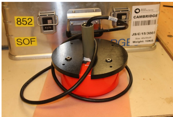
Figure 5-6: Re-terminated potting of cable and transducer
