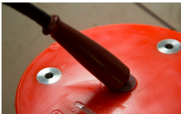
Figure 5-5: Broken termination of cable entering WBAT transducer
