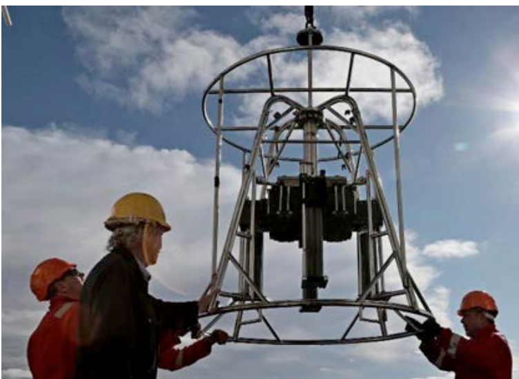
Figure 9.1.1. Deployment of megacorer with 4 tubes
