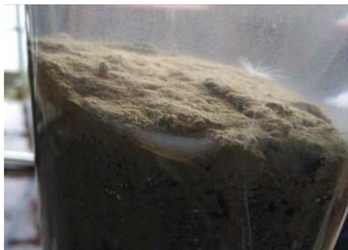
Figure 9.1.2. Intact sediment-water interface with benthic fauna in a Megacorer tube
