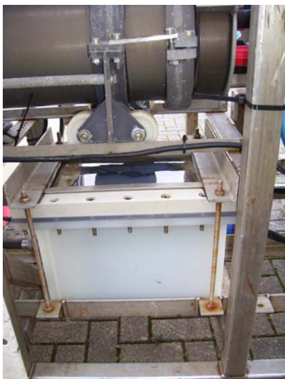
Figure 14. The main pressure compensated power transformer housing, situated just under the main pressure tube.
