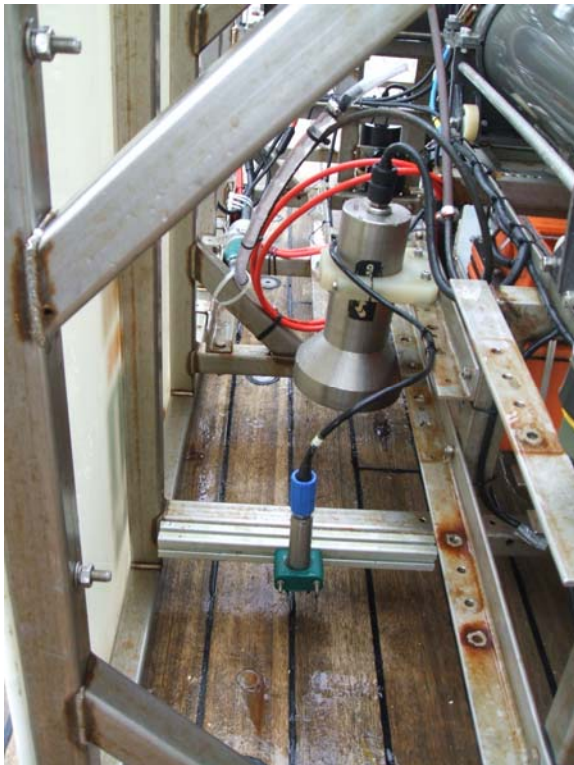
Figure 13. View from the rear of the SHRIMP frame showing the downward facing BOWTECH camera (foreground) and the larger silver pressure vessel holding the domestic camcorder.
