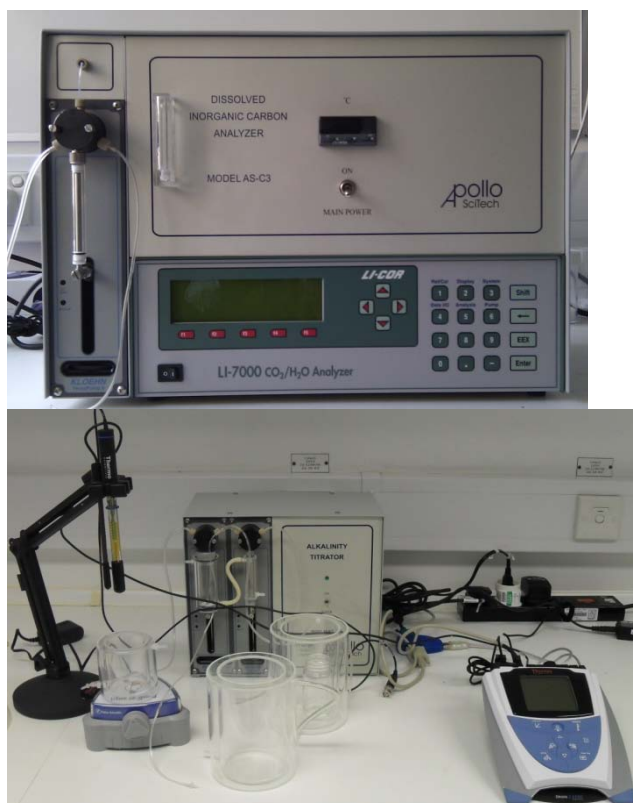
Figure 1. Apollo AS-C3 (left) and AS-ALK2 (right) used for the determination of Dissolved Inorganic Carbon and Total Alkalinity.
