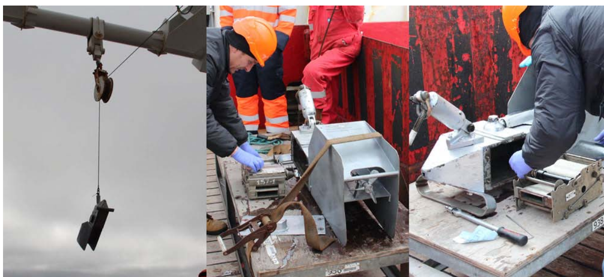
Plate 3: Recovery of CPR and winding-on of the internal mechanism
