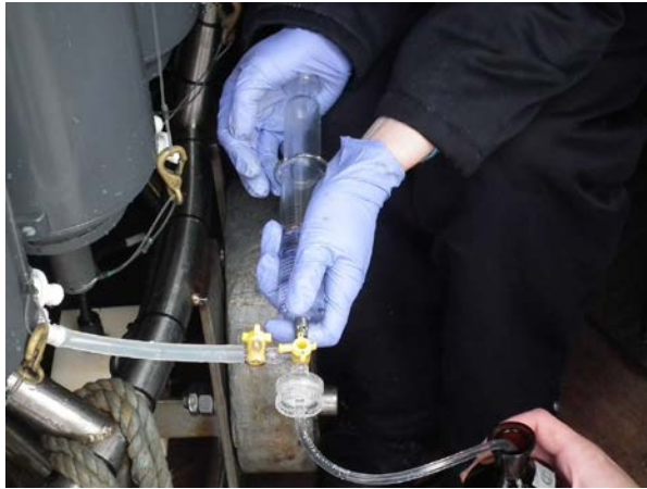
Figure 7.2. Sampling water for trace gas analysis from CTD casts
