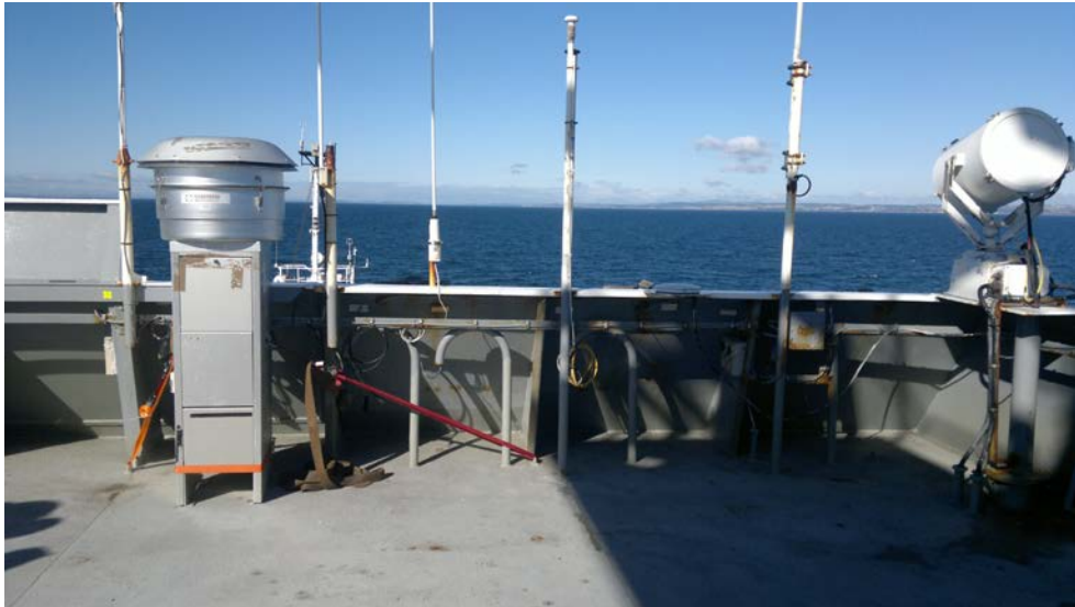
Figure 8.1. Location of the aerosol collector on the monkey island deck of RRS James Clark Ross during cruise JR288.
