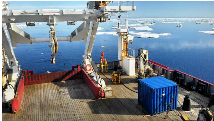
Figure 3.1: VMP 500 setup on aft deck port side, with hydraulic line puller (left), winch (middle) and 6ft container(right) housing hydraulic powerpack and data recording laptop.
