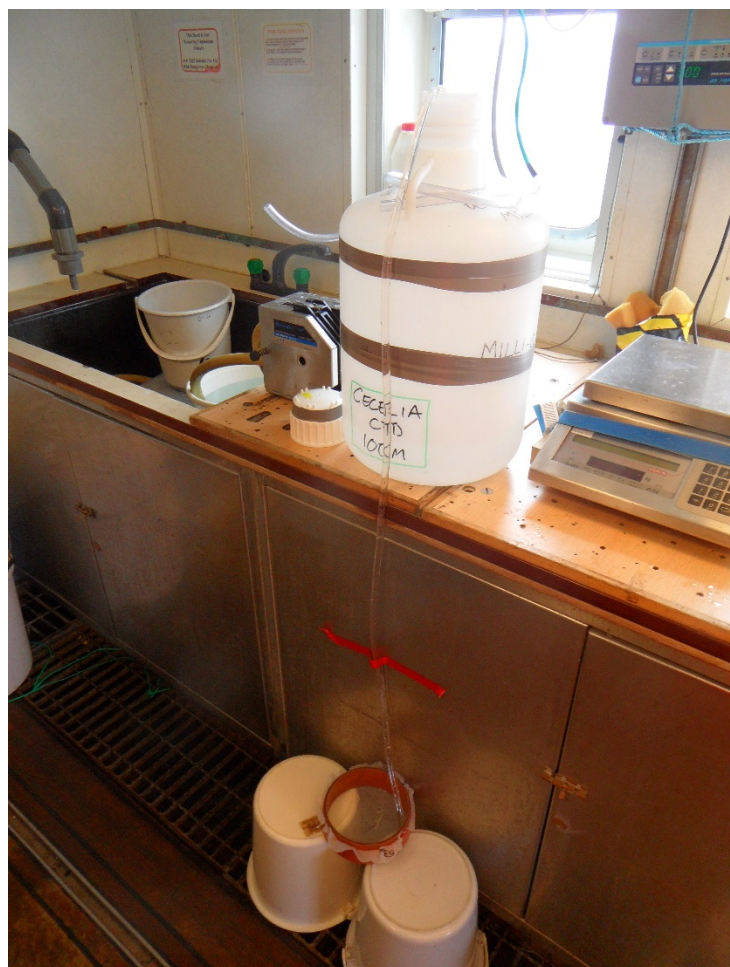
Figure 7-25: Set-up of siphoning system to decant CTD water from carboys to filter
