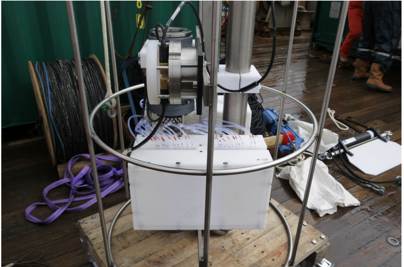
Figure 4-6: Aquamonitor just prior to deployment on deep water mooring
