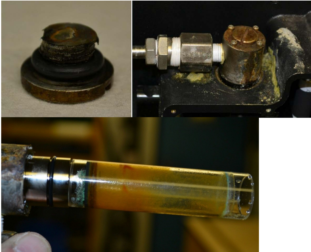
Figure 9-2: Views of the worn parts on the oceanlogger Turner fluorometer
