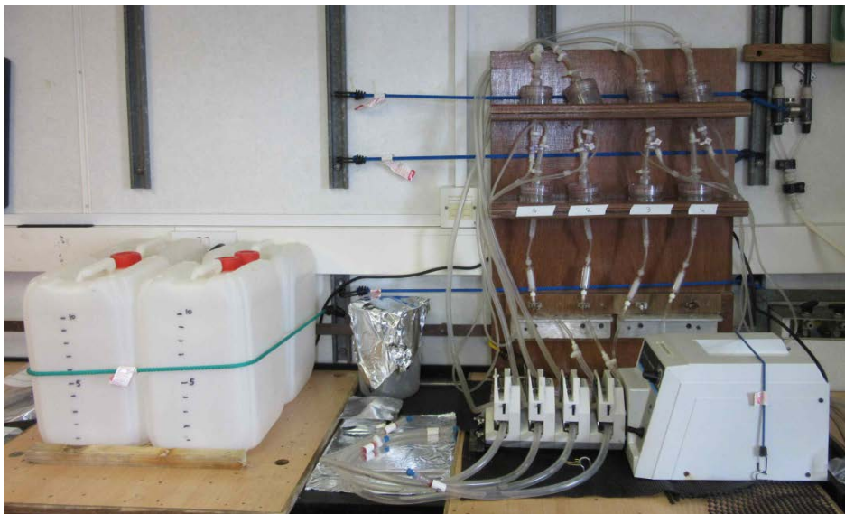
Figure 7-11: In-line filtration system.
