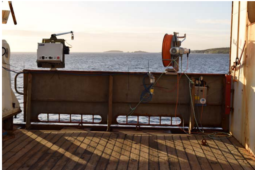
Figure 12.1: (clockwise from top left) View of various sensors on the nose of the MSS probe, the electric winch, and its location on the stern rail.
