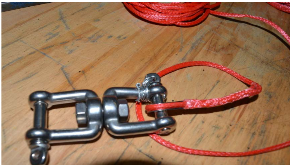
Figure 7.3. 12mm Swivel and 3.5mm Dyneema tether attached to each buoy.
