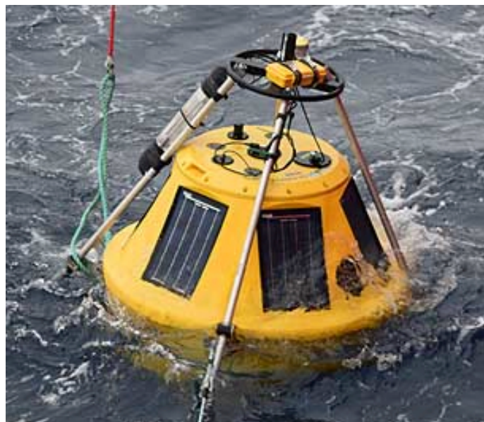
Figure 8.1. Wave buoy with externally-mounted radar reflector, light and waterproof case containing GPS and satellite communication cards.
