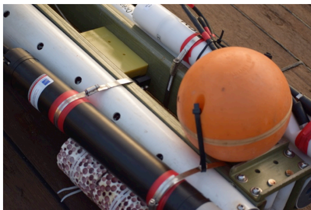
Figure 8.7. Wirewalker with attached CTD, Aquadopp and extra buoyancy.
