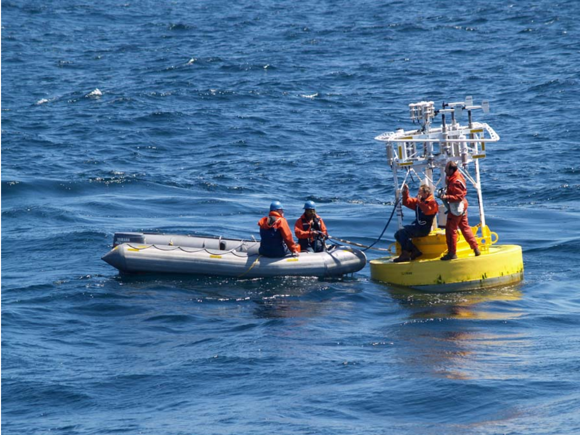
Sensor repair work underway on the CLIMODE surface buoy.
