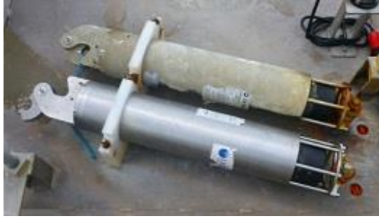
Figure 26: IXSEA Acoustic Releases within the frame
