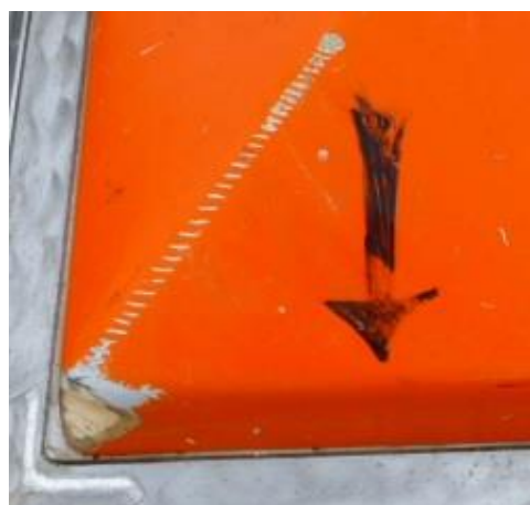
Figure 25: Trawl wire damage to frame
