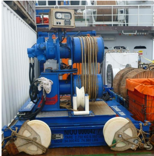
Figure 19: NIOZ LEBUS Double Barrel Winch
