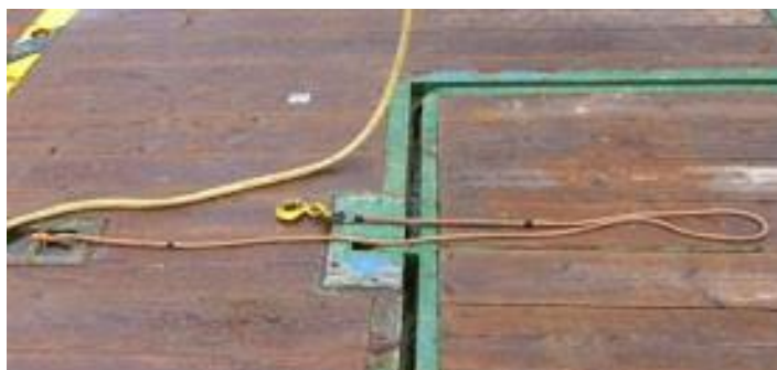
Figure 18: Deck stopper used for all moorings
