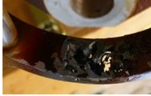
Figure 27: Sever corrosion of the A/R top plate
