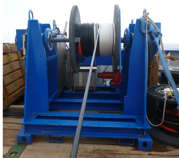
Figure 20: Spooling Winch used with the DB winch
