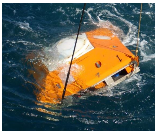
Figure 24: Recovery of the Trawl proof frame
