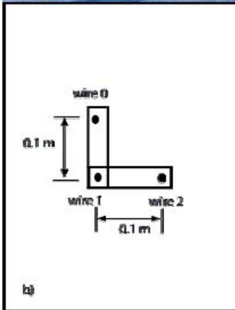
Figure 35 a) The wave buoy deployed in the Mull of Kintyre during day 312 and b) the configuration of the three wave wires (looking from above).
