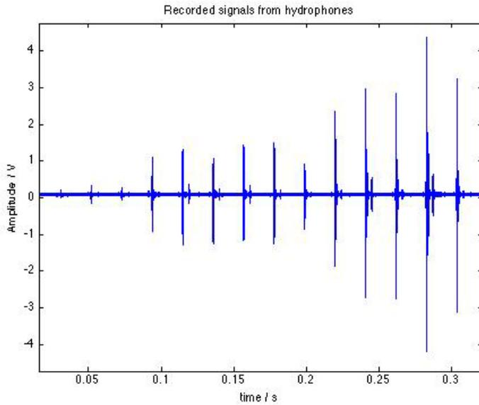
**Figure 36.** Measured pulses from the acoustic system. 14 pulses can be seen in the recording, each pulse increasing in frequency. The pulses are 1 ms long and separated by 20 ms. Recordings from different hydrophones can be compared to measure attenuation and this information can be used to calculate the bubble population.
