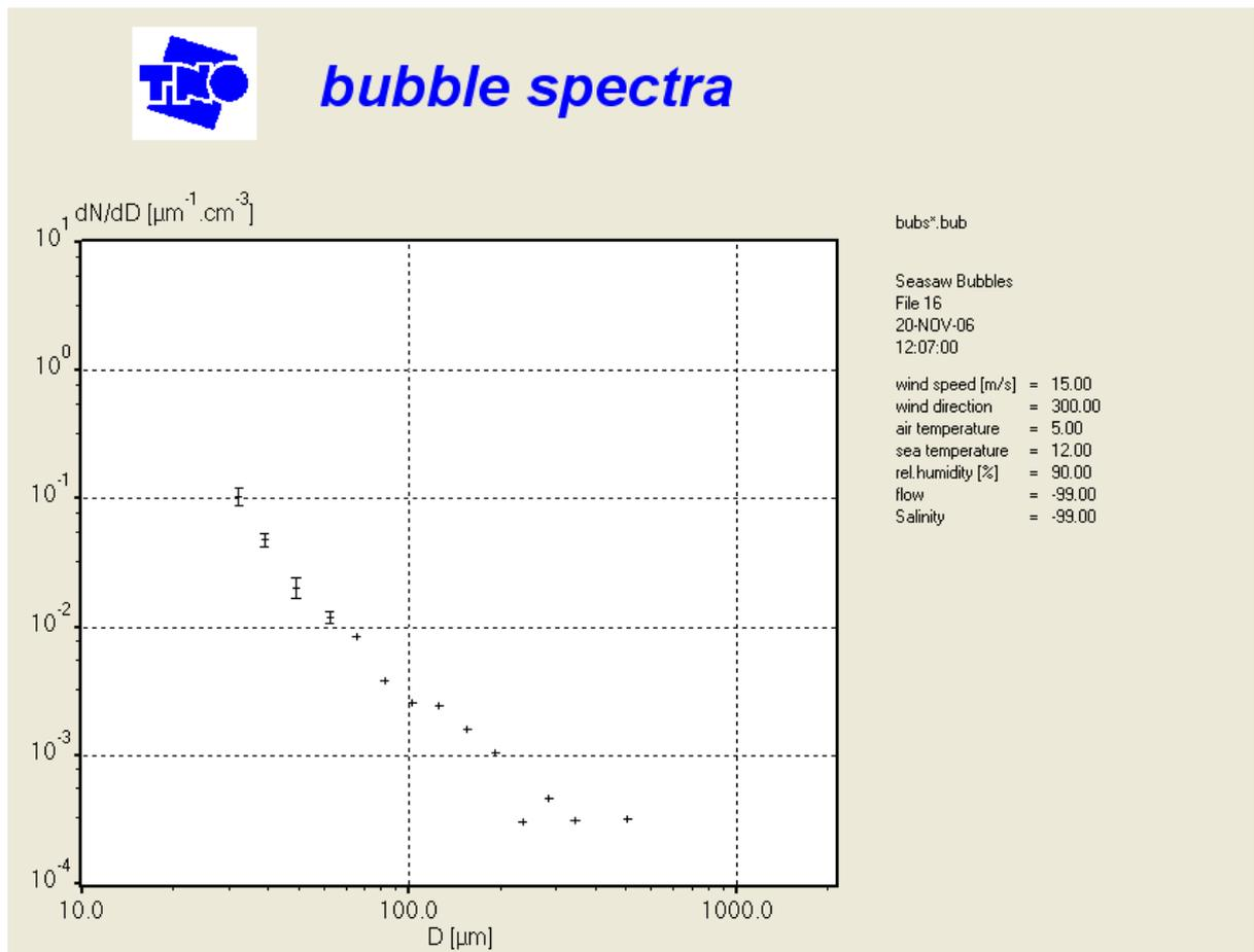
**Figure 50.** Bubble size spectrum
