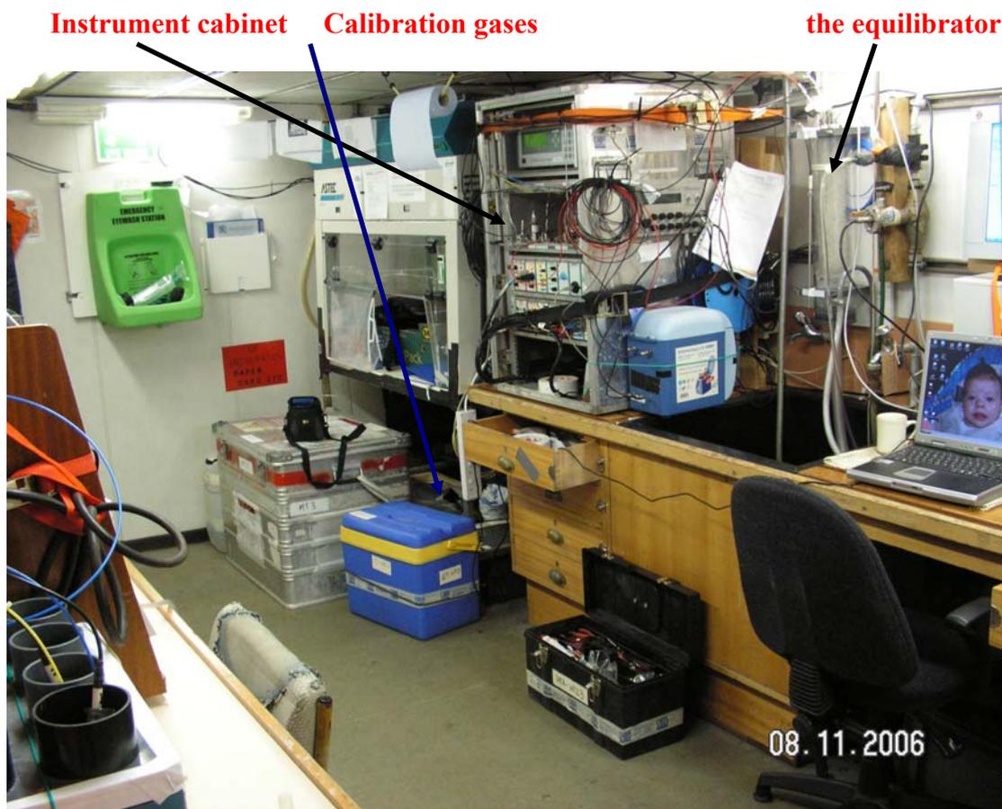
**Figure 40.** The CO<sub>2</sub> instrumentation as installed during D313.
