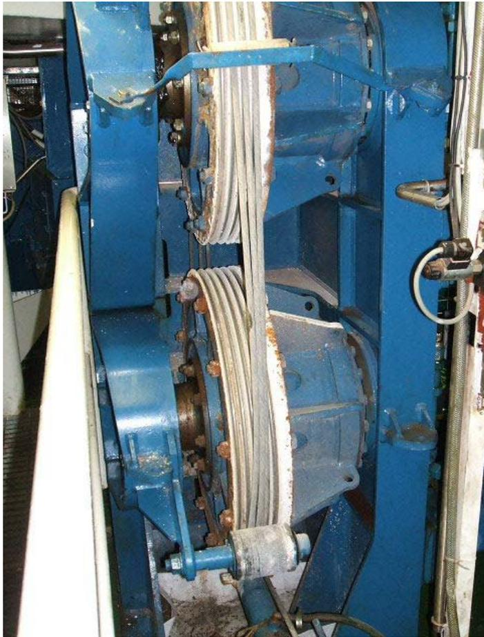
**Traction wires in place**
