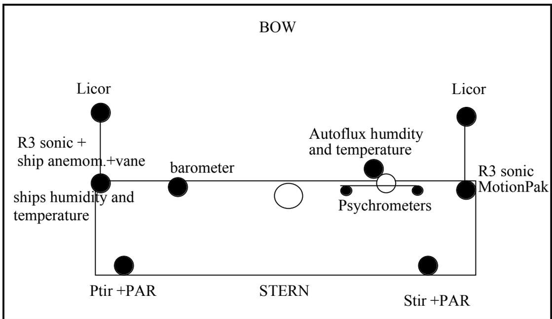
**Figure 23.** Schematic plan view of the foremast platform, showing the positions of the sensors.
