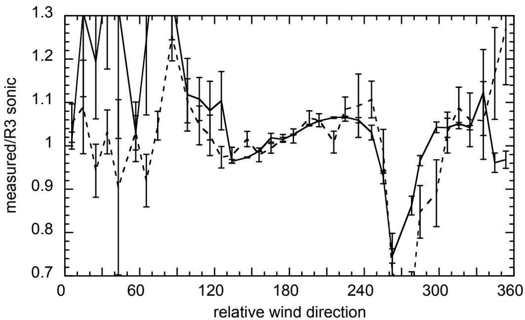
**Figure 24.** Measured wind speed / wind speed from the R3 sonic, MR3 sonic (bold line) and ship's anemometer (dashed line) each binned against relative wind direction. Only open ocean data is displayed and error bars indicate the standard deviation of the mean. A relative wind direction of 180 degrees indicates a flow directly on to the bow of the ship.
