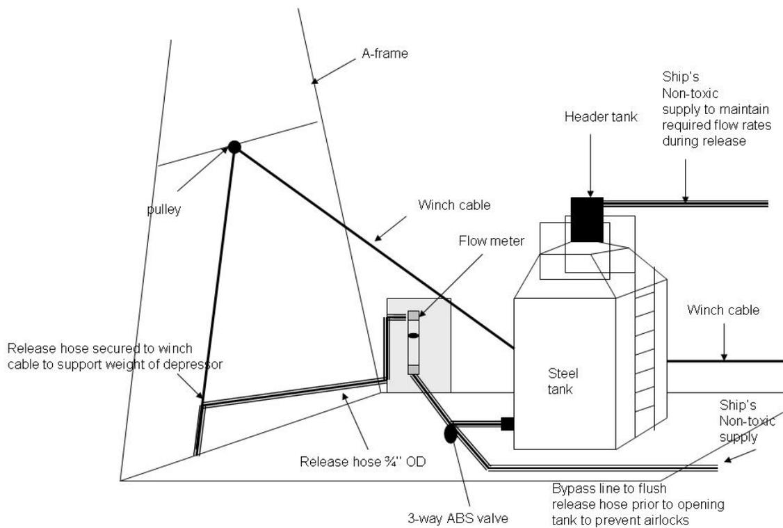
**Figure 8.** Schematic detail of tank, hosing and water supply during release of  $^3\text{He}$  and  $\text{SF}_6$
