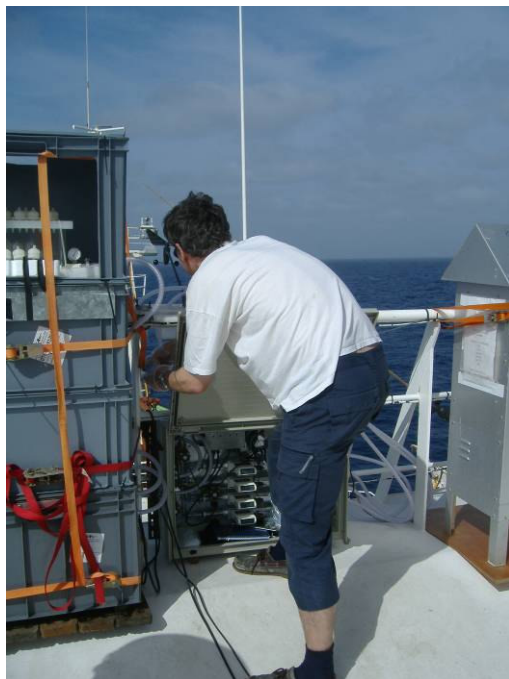
Figure 2. The aerosol sampler on the monkey island
