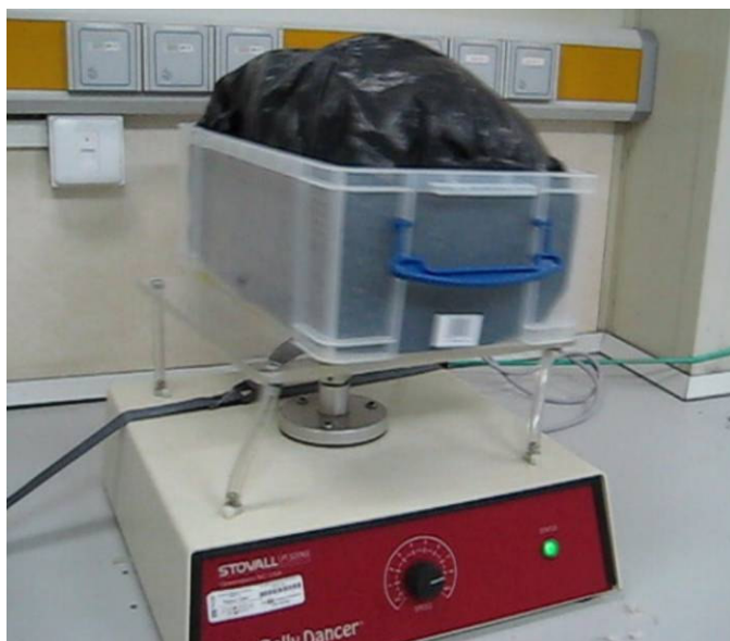
Figure 3. The dust dissolution experiments. Agitation of dust containing seawater samples.
