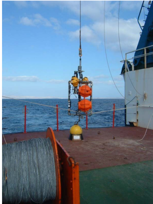
b – Wire test frame before deployment with LinkQuest and Benthos acoustics attached and a Seabird MicroCAT
