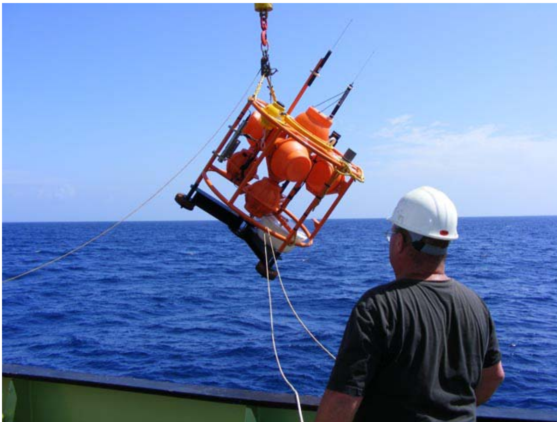
Figure 43 Benthic Lander (Mini-MYRTLE) deployment 1
