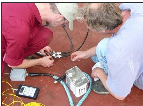
Figure 14 Joe Garrard (HydroLek contractor) and Lee Fowler (NOCS) work on the fibre optic connections inside the umbilical termination bottle
