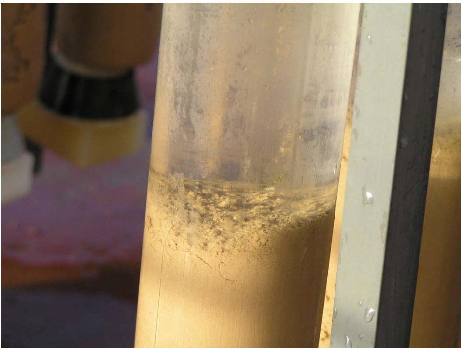
Figure 36 Detail of sediment water interface showing very little disturbance
