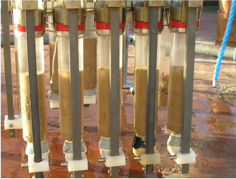
Figure 35 Image of multicore samples showing all tubes had penetrated and sealed successfully
