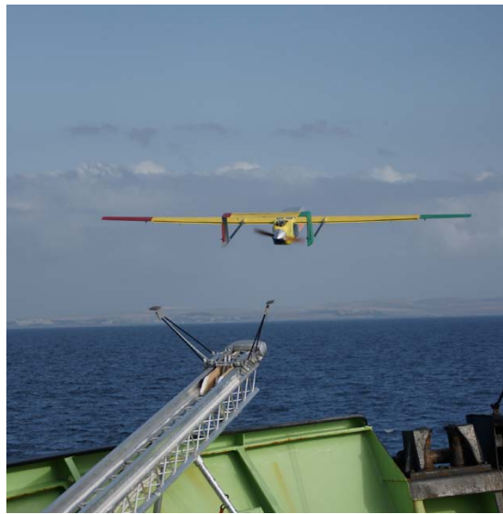
Figure 68 - Launch of the UAV
