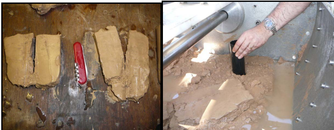
Figure 19 HyBIS Sediment sample taken using an improvised push core. Results of push cores: minimally disturbed sediment profiles.
