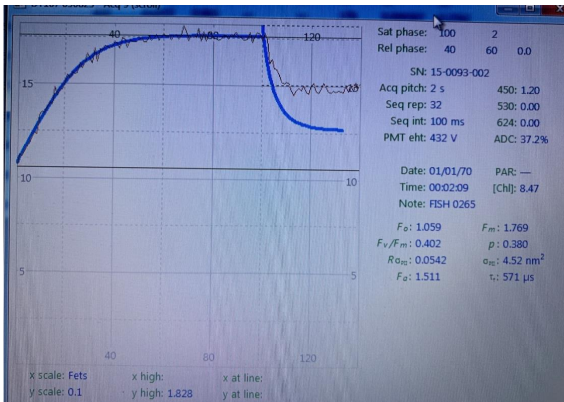
Figure 6.1 Summary of measurement conditions, including PMT eht, and an example of the fluorescence scans (FISH 0265).
