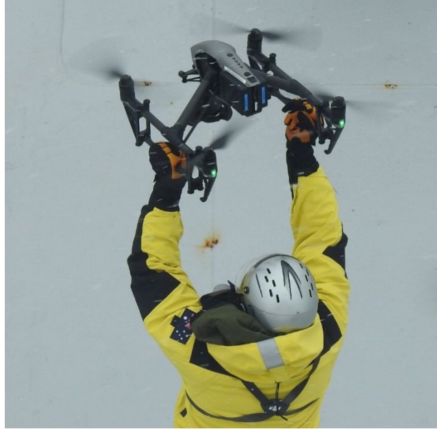
The DJI Inspire 2 ('media') UAV used to collect scientific data and general whale and scenic imagery. © Peter Shanks, MNF.
