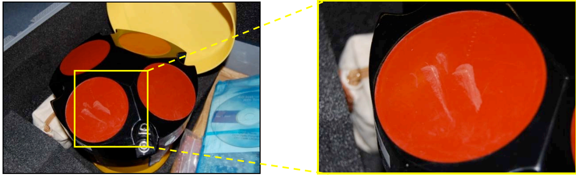
Figure 40: Damage to the LADCP
